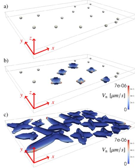
**Figure 3.5:** 3D simulation of the XRMON-SOL experiment. a) initial configuration with the seeds,  $t_{\text{sim}} = 0$ , b)  $t_{\text{sim}} = 50$  s, and c)  $t_{\text{sim}} = 130$  s. The color map indicates the normal growth velocity of the envelopes,  $V_n$ .
