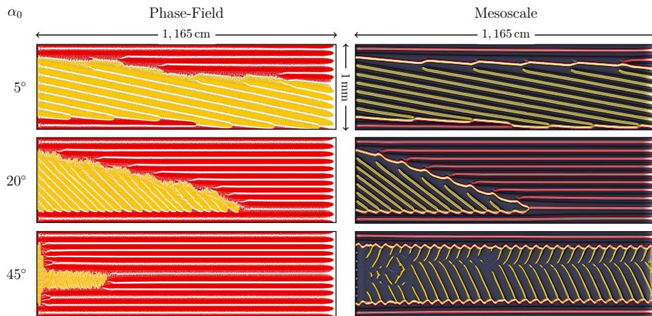
**Figure 3.15:** Spatiotemporal plots of growth competition predicted by the phase-field (left) and the mesoscopic model (right). The well-oriented grains are shown in red and the grain misoriented by the angle  $\alpha_0$  is shown in yellow (full for phase field, contour for mesoscale where solid fraction is superimposed). Note that the horizontal length is displayed compressed by a factor of 0.3.
