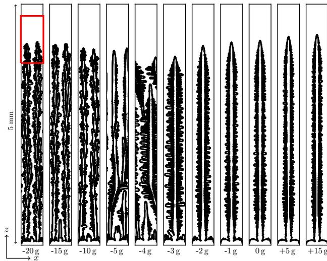
**Figure 3.18:** Columnar microstructure at different gravity levels predicted by the phase-field model. Spatiotemporal plots of the solid-liquid interface after 200 s are shown. At positive gravity, the gravity vector is oriented in the growth direction, at negative gravity it is opposite to the growth direction. The red rectangle represents the moving calculation domain.
