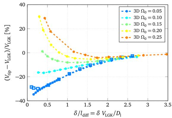
**Figure 3.22:** Dependence of the relative error of the predicted primary tip speed on the normalized stagnant film thickness,  $\delta/l_{\text{diff}}$ .
