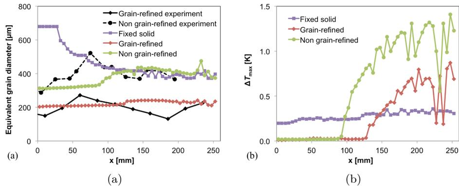
**Figure 2.11:** Predictions of the grain size profile across the ingot thickness. (a) Profiles of equivalent grain diameter. (b) Profiles of maximum undercooling as an indicator of the activation of inoculant particles.
