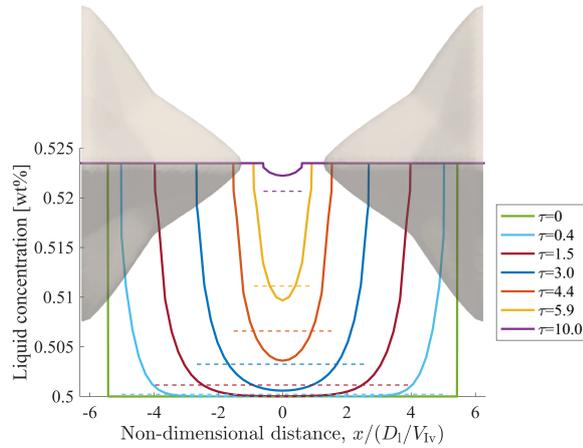
**Figure 4.2:** Profiles of liquid solute concentration between the primary tips of two dendrites growing towards each other (solid lines) and average concentration in the whole extragranular liquid volume (dashed lines). Different curves show the profiles at different times. The grains are arranged periodically in a BCC arrangement.
