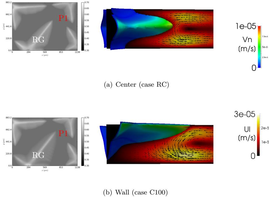
**Figure 3.8:** The influence of natural convection on the primary arm growth in a thin sample depends on the grain position: (a) grain in the center of the sample thickness; (b) grain at the top wall. Left: simulated X-ray radiographs. Right: envelope growth velocity,  $V_n$ , and liquid velocity,  $U_l$ , in a plane perpendicular to the  $x$ - $y$  plane and containing the grain center and the tip P1.
