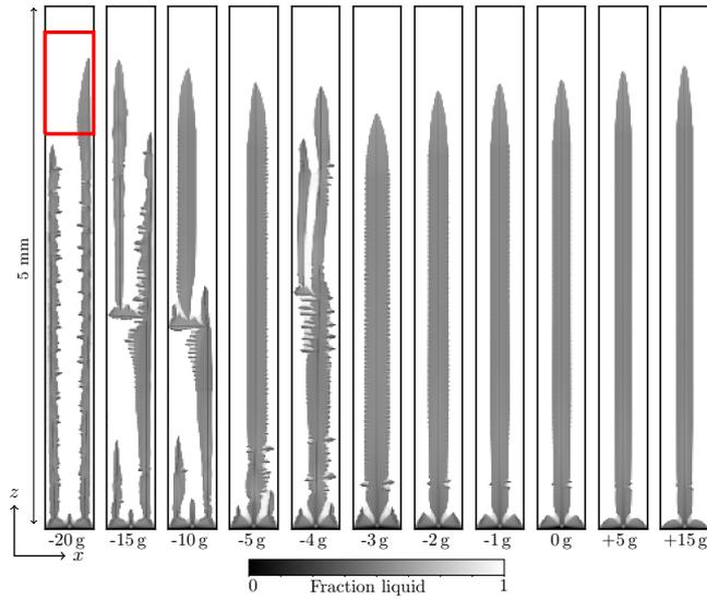
**Figure 3.17:** Columnar microstructure at different gravity levels predicted by the mesoscopic model. Spatiotemporal plots of the solid-fraction field after 200 s are shown. At positive gravity, the gravity vector is oriented in the growth direction, at negative gravity it is opposite to the growth direction. The red rectangle represents the moving calculation domain.
