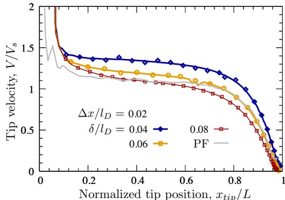
**Figure 3.23:** Evolution of the primary dendrite tip velocity for  $\Omega_0 = 0.05$  from GEM simulations compared to phase-field. The influence of the stagnant-film thickness,  $\delta$ , on the velocity transient is shown. The final length of the primary arm,  $L$ , is two times the diffusion length,  $l_D = D_1/V_{\text{tip}}$ , where  $V_{\text{tip}}$  is the steady-state tip speed.
