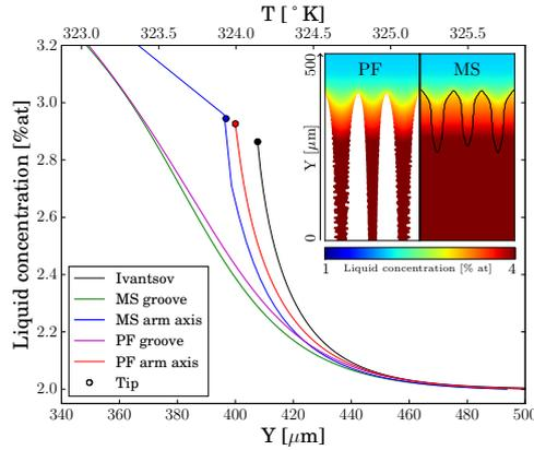
**Figure 3.12:** Liquid concentration profiles along the axis of a primary arm and along a groove between two arms. Comparison of a phase-field and a mesoscopic simulation in steady-state growth. The Ivantsov solution for a free tip growing at the pulling speed is also shown for comparison. The inset shows the full concentration fields from the phase-field (PF) and mesoscopic (MS) simulations, the envelope of the mesoscopic model is shown as a black line.
