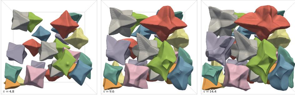
(b) 27 grains with a mean distance of  $\bar{d}_{cc} = 11 l_{\text{diff}}$  ( $N_V^{\text{ldiff}} = 10^{-3}$ ).
