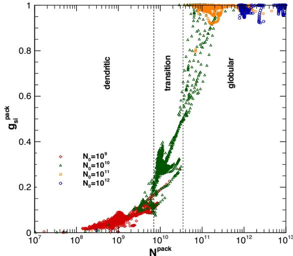
**Figure 2.4:** The final grain morphology in dependence of the local grain density. The trend is constructed from a compilation of results in all mesh points from four computations with different nucleation densities  $N_0$ . The grains are dendritic for  $g_{\text{si}}^{\text{pack}} \ll 1$  and globular for  $g_{\text{si}}^{\text{pack}} \rightarrow 1$ .
