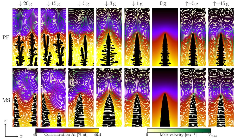
**Figure 3.19:** Columnar dendrite growth in Ti-45 at.%Al as function of gravity level for the phase field (PF) and the mesoscopic model (MS). Flow streamlines are superimposed onto concentration maps. Note that the maximum velocity magnitude  $V_{\max}$  is different for each frame.
