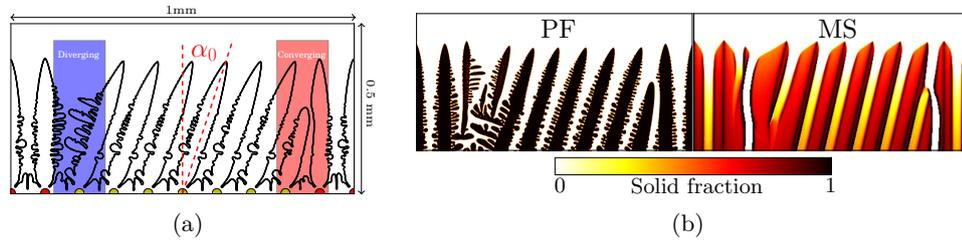
**Figure 3.14:** (a) Schematics of the prototype configuration for grain competition, the grain inclination angle,  $\alpha_0$ , and the calculation domain. (b) Snapshot of the growing dendrite structure given by the phase-field (PF) and by the mesoscopic model (MS) for  $\alpha_0 = 20^\circ$  for the same physical time.
