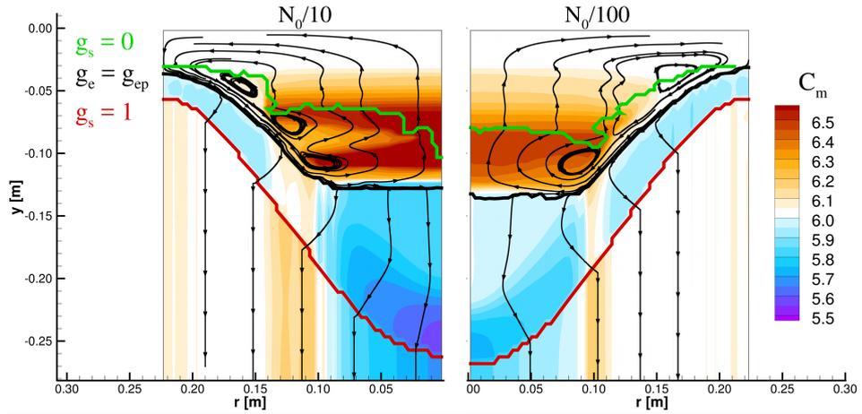
**Figure 2.8:** The influence of the morphology transition on the macrosegregation. Flow and fields of the average copper composition in the liquid and the solidification zone. Left:  $N_{ino} = N_0/10 = 0.1$  kg/t, which gives globular grains. Right:  $N_{ino} = N_0/100 = 0.01$  kg/t of grain refiner, which gives dendritic grains.
