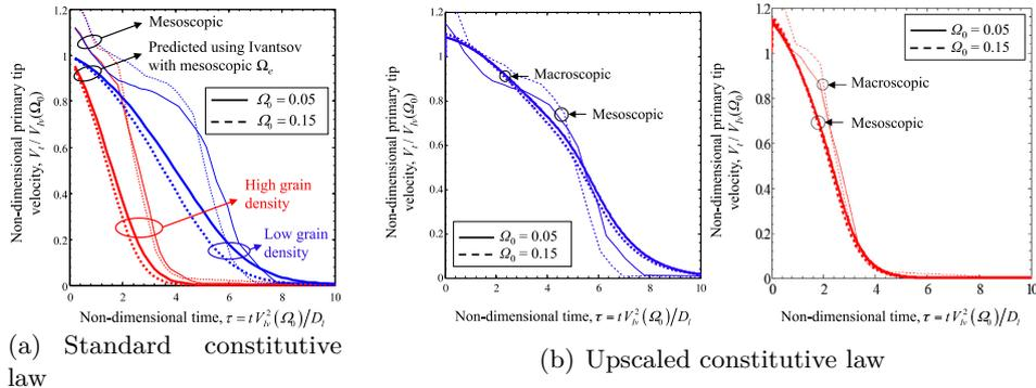
**Figure 4.3:** Comparison between mesoscopic primary tip velocities and primary tip velocities obtained with macroscopic constitutive laws. (a) Standard constitutive law that gives the Ivantsov primary tip velocities corresponding to the *average* supersaturation in the extragranular liquid. (b) New upscaled constitutive law that uses an effective supersaturation.
