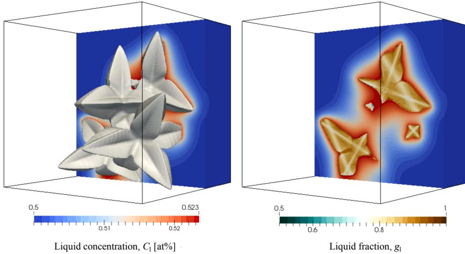
**Figure 3.1:** Example of results of a simulation with the mesoscopic model. Left: four interacting equiaxed grain envelopes. Right: a slice across showing the liquid fraction field in the interior of the envelopes and the concentration field in the liquid outside the envelopes.
