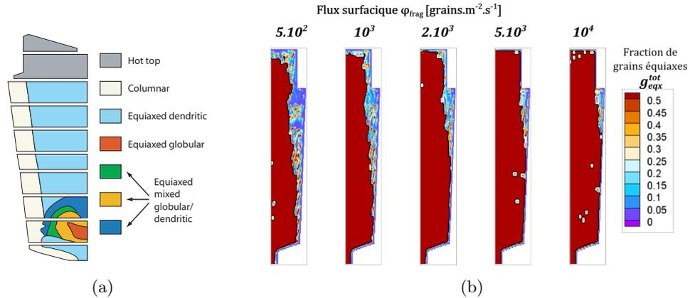
**Figure 2.6:** CET in the 3.3 ton ingot. (a) Experimental characterization of the macrostructure. (b) Model prediction of the CET assuming dendrite fragments from the columnar zone as the only source of equiaxed grains. The shape of the columnar zone depending on the flux of the fragments at the columnar front [fragments/(m<sup>2</sup> s)] is shown.
