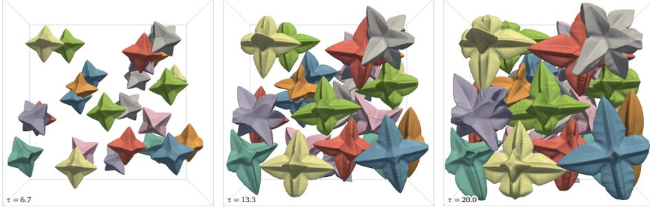
(a) 27 grains with a mean distance of  $\bar{d}_{cc} = 22 l_{\text{diff}}$  ( $N_V^{\text{ldiff}} = 1.25 \cdot 10^{-4}$ ).
