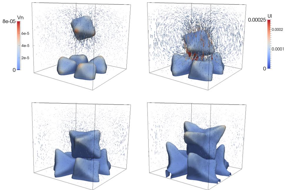
**Figure 3.25:** Simulation of settling and growth of an equiaxed Al-4%Cu grain and packing on a layer of packed grains. The color of the envelope surface shows the envelope growth velocity [m/s]. Arrows show liquid velocity vectors colored by speed,  $U_l$  [m/s].
