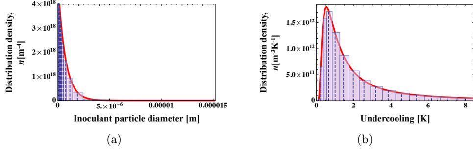
**Figure 2.10:** Distribution density function of the inoculant particle population with respect to the particle size (a) and activation undercooling (b), for an Al-5Ti-1B grain refiner added at 5 kg/t.
