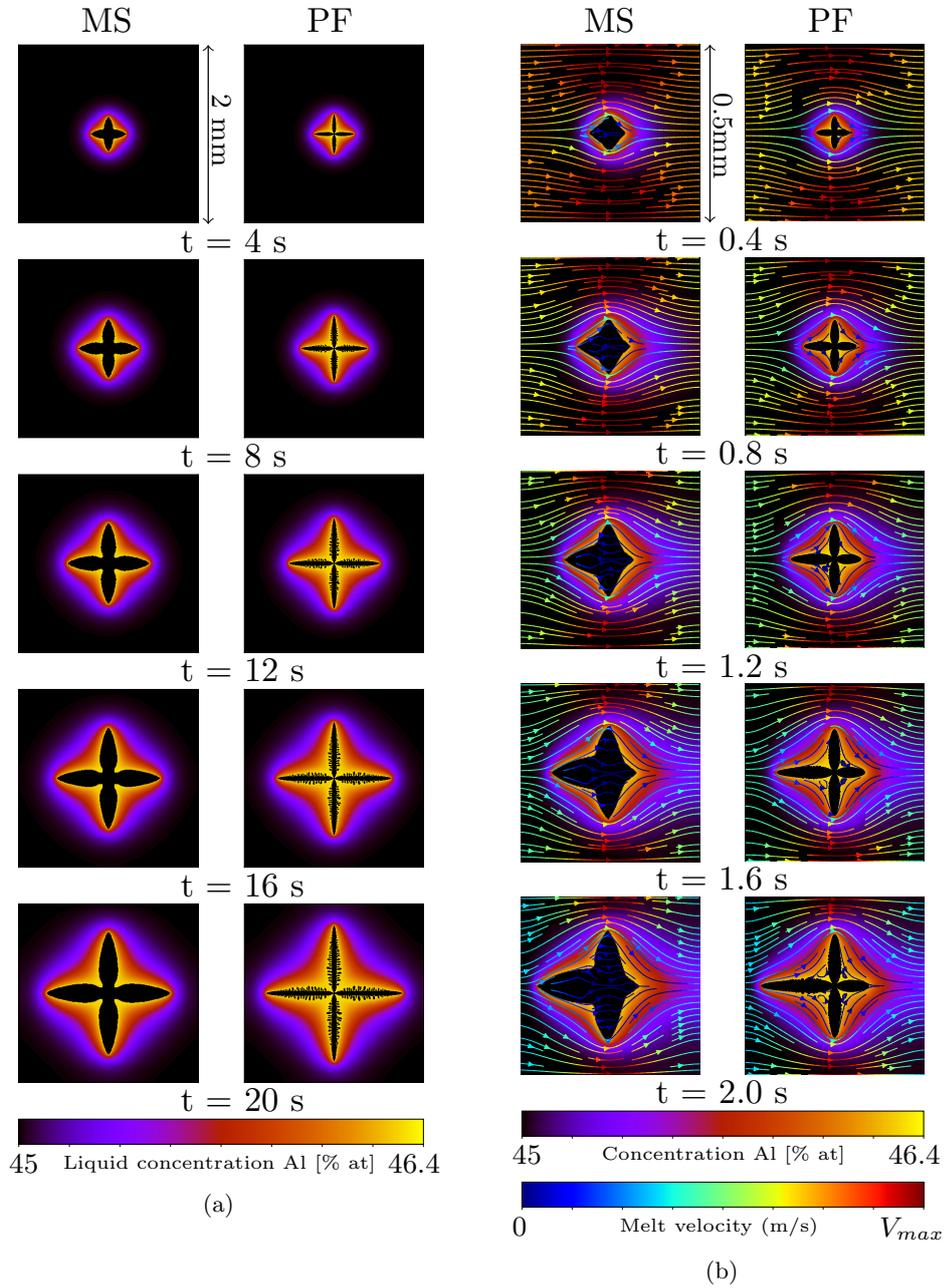
**Figure 3.10:** Evolution of the equiaxed grain during (a) purely diffusive growth and (b) growth in a forced flow. Simulations by the mesoscopic envelope model (MS) and by the phase field model (PF). Fields of liquid concentration, streamlines, dendrite envelope (MS), and solid-liquid interface (PF) are shown.
