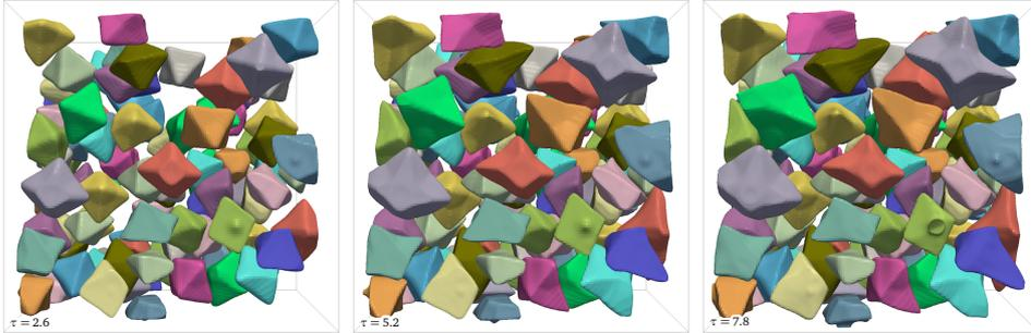
(c) 108 grains with a mean distance of  $\bar{d}_{cc} = 7 l_{\text{diff}}$  ( $N_V^{\text{ldiff}} = 4 \cdot 10^{-3}$ ).
