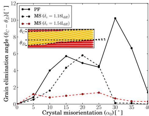
**Figure 3.16:** Grain elimination angles as function of the crystal misorientation angle  $\alpha_0$  of the misoriented grain. Comparison between mesoscopic (MS) simulations for two stagnant-film thicknesses and the phase-field (PF) simulations. Note that the stagnant-film thickness is specified in terms of the steady-state diffusion length,  $l_{diff} = D_1/V_{pull}$ , where  $V_{pull}$  is the pulling speed of the directional solidification.
