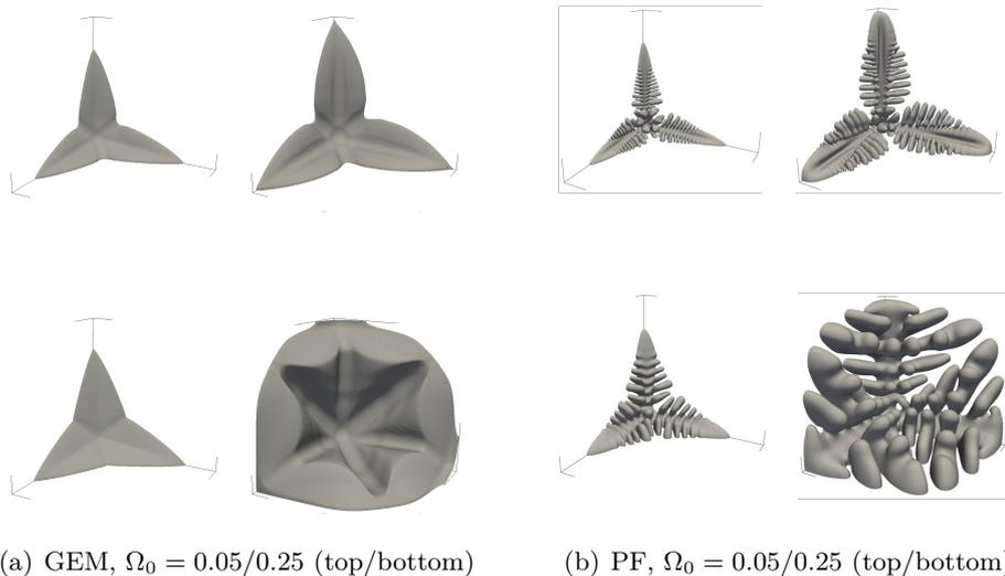
**Figure 3.11:** Evolution of the grain shape (1/8 of an equiaxed dendrite) during isothermal equiaxed growth with interaction (in a cubic confinement). Comparison of the grain envelope model (GEM) and the phase-field model (PF) for two different supersaturations,  $\Omega = 0.05$  and  $0.25$ . (phase-field images courtesy of Damien Tournet, IMDEA Materials).
