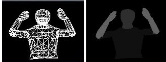
Figure 2-19: Rendering the 3D model: The left image is the generated 3D model pose and the right image is the model projection with the body segments flat-rendered according to their three color labels (arms, head and clothes).
