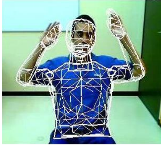
Figure 3-3: Calibrating and initializing our 3D model with respect to the actor in the first input image.
