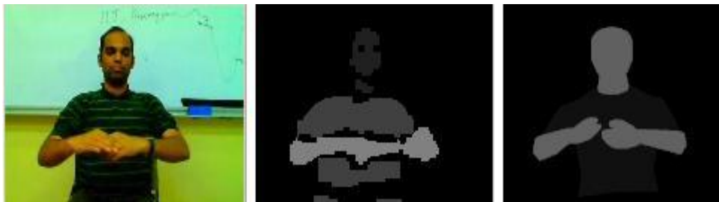
Figure 3-7: The limited accuracy of region-based registration. The images are respectively: the captured image, the segmented image and the projection of the registered 3D human body model after optimization. The pose of the 3D model differs from the pose of the actor because the region-based registration is not accurate.
