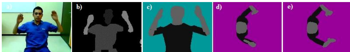
Figure 4-1: Monocular observation ambiguities: a) the input image, b) the segmented image, c) a model projection that matches the segmented image, (d) and (e) are different 3D poses that both match the segmented image as they give the same model projection in (c).
