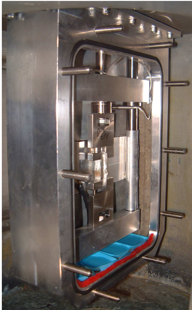
Figure 7.5: Left: Photograph of a silk sample (white fiber bundle in the center of the image) inside the humidity chamber for in situ tensile testing mounted inside the sample bay of the time-of-flight spectrometer IN6. The chamber (see also Fig. 7.4) is shown with the front cover removed. The force sensor is visible as a cylindrical metal structure on the upper center of the photograph with the signal cable arriving from the right. The neutron beam impinges on the sample horizontally, arriving from the right edge of the photograph. The blue plastic troughs at the bottom of the chamber contain pure water or saturated salt solutions, respectively, to define the humidity inside the chamber. The edge-to-edge distance between the steel hooks holding the fiber bundle is 3 cm. Right: Stress-strain curves obtained in situ during the IN6 experiment using the apparatus depicted in the left part of the figure (humidities see legend). TOF data have been recorded at the positions on the stress-strain curves marked by the capital letters and at \epsilon \approx 0 [143]. During these recordings the otherwise continuous tensile elongation was interrupted, resulting in the observed relaxations in the tensile stress \sigma . The solid lines are linear fits to determine the mechanical moduli. (Figure from [143])
