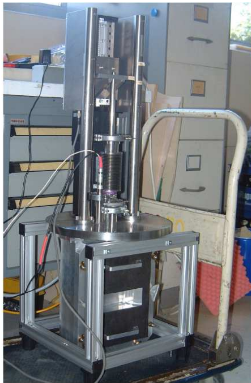
Figure 7.4: Left: Photograph of the tensile machine for in situ neutron scattering experiments on fibre materials (see also figure 7.5). The humidity chamber holding the sample is at the bottom. The black neutron-absorbing B_4C cover leaves a rectangular entrance window for the neutron beam. The circular steel flange above the humidity chamber seals the tensile machine such that the humidity chamber is surrounded by the vacuum of the neutron spectrometer sample bay. Right: Schematic explaining some of the components of the tensile machine. The cylindrical adaptor to the spectrometer sample bay has been removed for the photograph. (Figure from [87])
