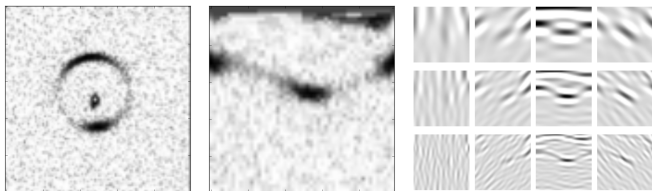
Fig. 2. Example of our feature extraction procedure used to transform a ring. The image on the right shows the response of a set of Gabor filters after convolution with a polar transformed image of an Einstein ring. The strongest response is seen in the orientation perpendicular to the radial direction and at the frequency most closely matching that of the ring.
