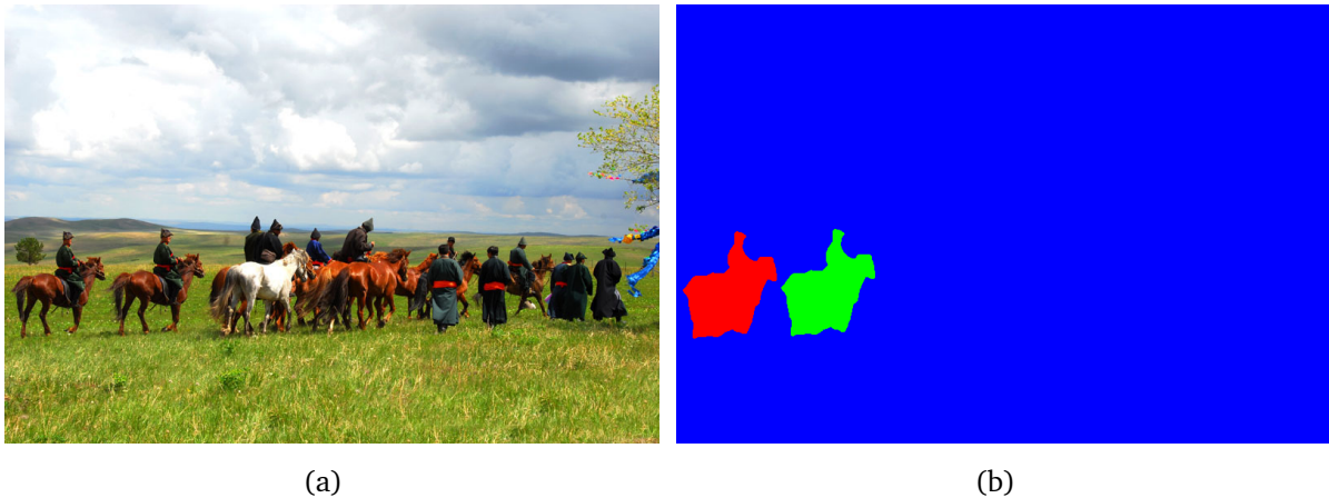
Figure 5.1 – Example of copy-move image from CASIA2 [DWT13] database. (a) The rider on the left has been copied. (b) Mask of the tampering, where green indicates the source area and red the target area of the copy-move.
