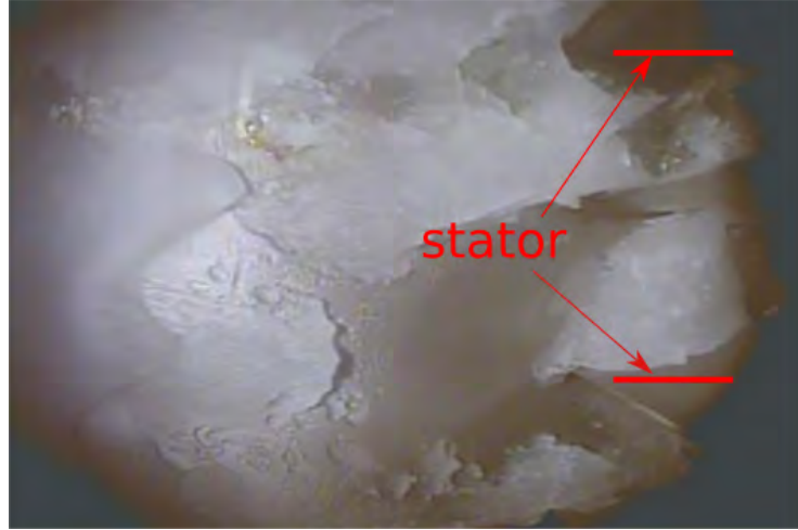
FIGURE 7.2. – Image of accretion at the second stator EGV trailing edge and on the Nozzle (upper duct wall) - Adapted from [153]
