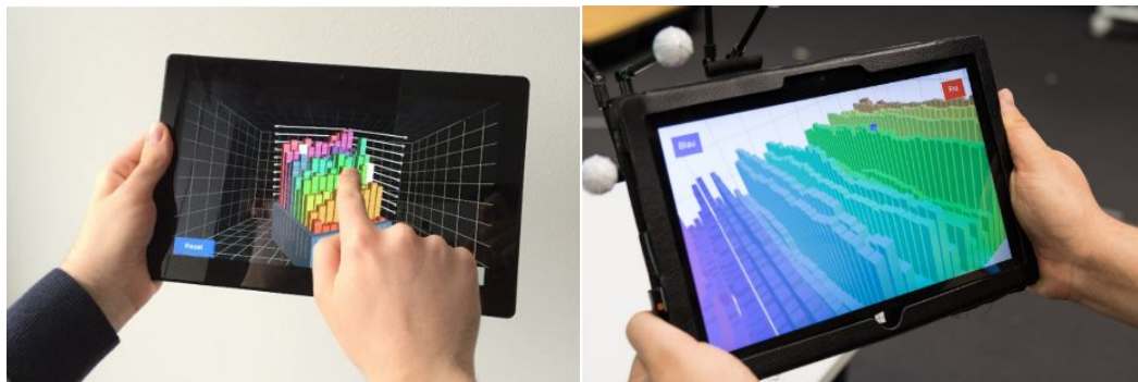
Figure 2.3.5: Bar chart visualization fixed on the mobile device (left) and in space (right). Source: Büschel et al. (2016).
