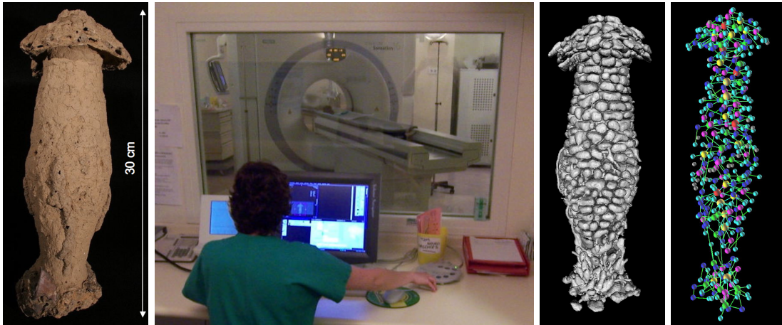
Figure 5.8 – (left) Photo of the epigeal part of a Cubitermes sp. nest. (middle left) The X-ray tomography control room with a protected view on the scanner. On this photo a Cubitermes acquisition is under way. (middle right) Virtual mold of the Cubitermes nest, representing the habitable space of the termites by rendering the walls invisible. (right) Network representation of the Cubitermes nest. The color of the nodes indicates their degree. Figs taken from the virtual nest museum .
