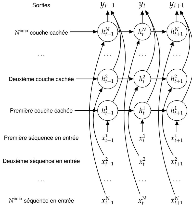
FIGURE 1.2 – Architecture LSTM parallèles (PLSTM) [Bouaziz, 2017].
