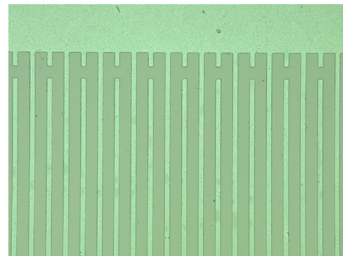
Fig. 10. Optical microscopy image of Ir 0.7 Rh 0.3 electrodes taken after the fifth 1 day-annealing process at 900 °C.
