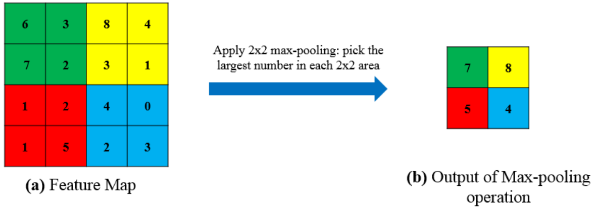
Figure 3.8 – An example of max-pooling operation. (a) is the output of convolution operation, (b) is the result after applying 2 \times 2 max-pooling operation. In typical CNN architectures, they use a window of 2 \times 2 (which is most common) because it provides the minimum spatial reduction of feature maps.
