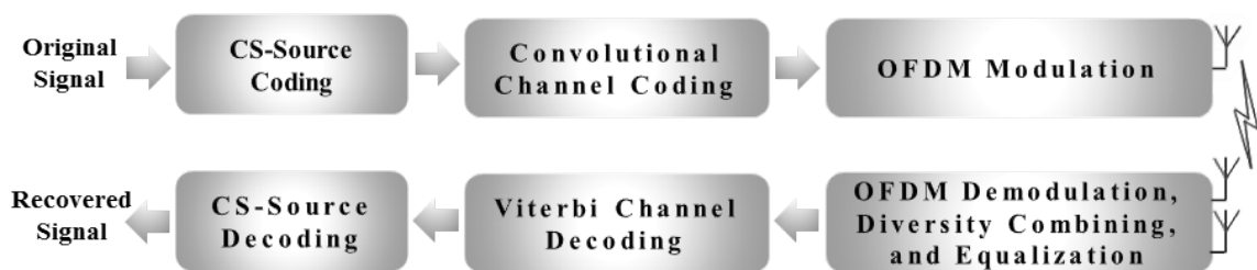
FIGURE 4.2: General diagram of the proposed communication scheme (note that this system integrates compressed sensing-speech coding instead of the current codecs standards such as G.722.2)
