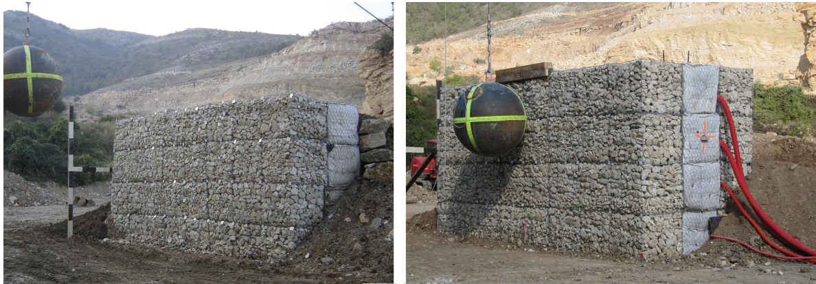
Figure 2.4 First and second type of real-scale structures, before impact (left and right, resp).
