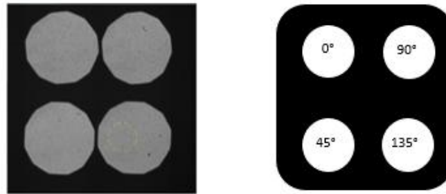
Figure 5.1 – All 4 channels from white paper. On the left, an example of raw data, on the right an illustration of the ideal 4 polarized detection channels. We can get the mean intensity value of each channel (i.e., measuring I_0 , I_{45} , I_{90} , and I_{145} ) to use in the G-factors. When working with tube lens TL=1.0x, we obtain a FoV diameter of 40\mu\text{m} .
