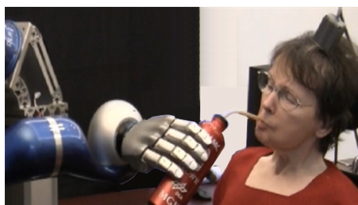
Figure 2.2 – Cathy Hutchinson used the BrainGate system to control a robotic arm with mental imagery alone. Here she picks up a bottle of water and drinks from it [Ven12]. Image credit: BrainGate.
