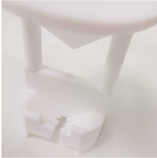
Figure VII.1: Picture of the KOH etching holder used for the patterned membrane recipe with Protek.
