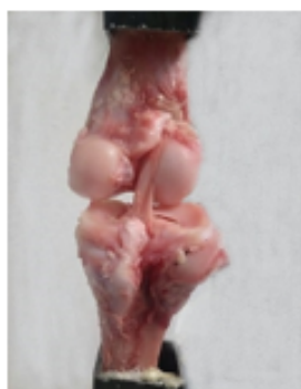
Figure 1: Biomechanical setup in caudal view of the CCL of an anatomical part included in metal support using resin.
