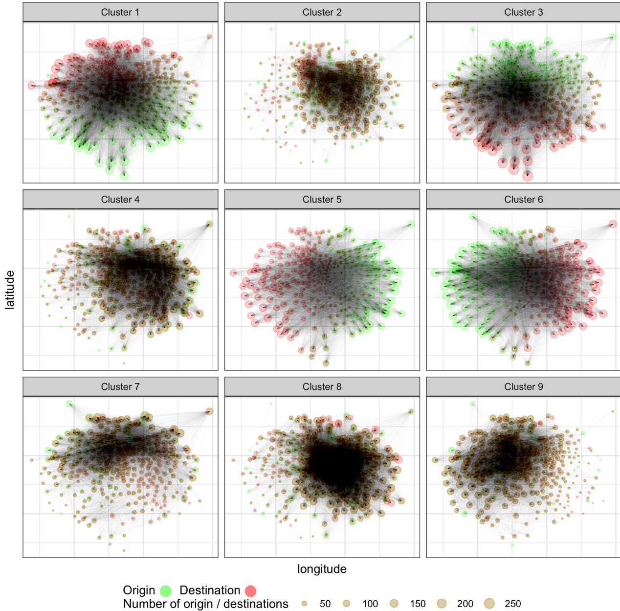
Figure 4.10: Origin-destination zones in each cluster. The clusters show differentiated geographical patterns. For example, clusters 1,3,5 and 6 represent trips that originate and terminate in the limits of the network and, thus, represent longer trips.
