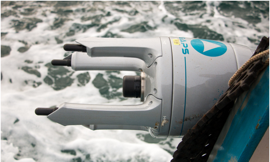
(a) USBL mounted on the mission boat. This device is made of four transceivers.
