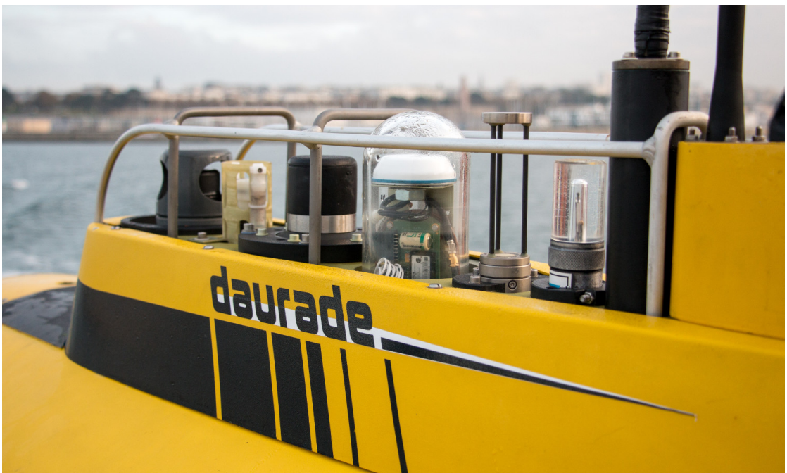
(b) The receiver unit is embedded on top of the AUV among other sensors.
