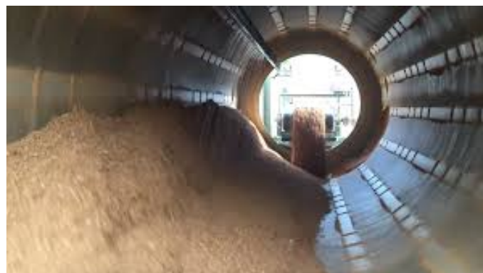
FIGURE 2 – Tambour de granulation.
