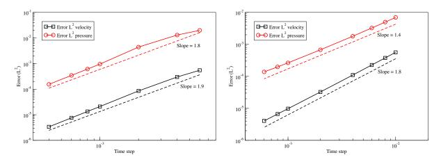
Figure 5.4: Time convergence rates with the standard incremental scheme (left) and the rotational scheme (right) at  $t^* = 1$  with K = 1 and p = 18 with the proposed open boundary conditions and spectral element method.
