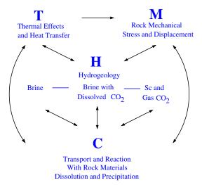
Figure 10.1: Coupled THMC processes, coupling thermal (T), hydrological (H), rock mechanical (M) and chemical (C) effects for geological storage of CO<sub>2</sub> (adapted from [226]).
