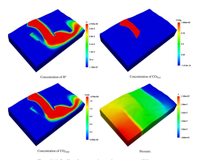
Figure 9.16: Profiles of concentrations and pressure at t = 1500 years.
