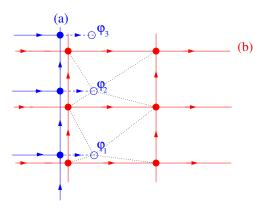
Figure 6.3: New stencil to ensure incompressibility constraint.
