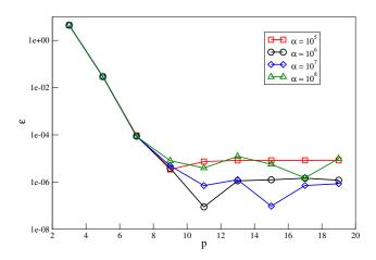
Figure 3.4: Convergence plots obtained using the penalty method for the first Stokes mode ( $\lambda^2 = 13.086172791$ ) as a function of the polynomial order p for several values of  $\alpha$ .
