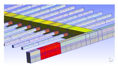
Figure 9.3: Grid of the module for UM1 (188 298 elements).
