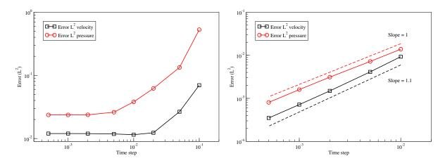
Figure 5.1: Time convergence rates with the standard incremental scheme (left) and the rotational scheme (right) at  $t^* = 1$  with K = 1 and p = 18 with standard open boundary conditions and spectral element method.
