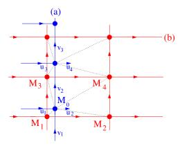
Figure 6.1: Interpolation of the pressure.
