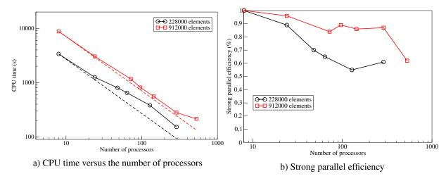
Figure 9.17: CPU time and strong parallel efficiency as a function of the number of processors.
