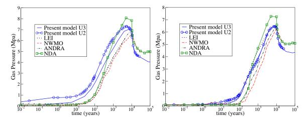
Figure 9.6: Comparison of the gas pressure. Left: P-C50-3 in the main drift. Right: P-Pd-1 in the bentonite of the access drift.
