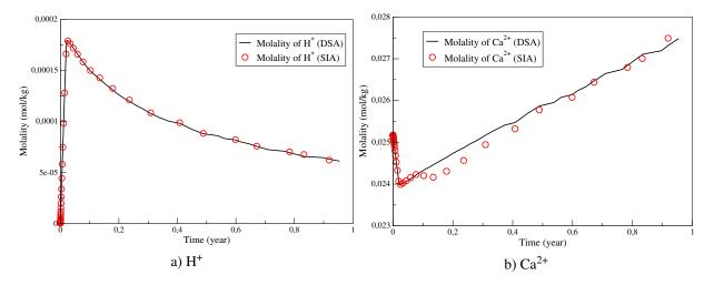
Figure 9.11: Comparison of the molalities of H<sup>+</sup> and Ca<sup>2+</sup> obtained with the DSA and the SIA.
