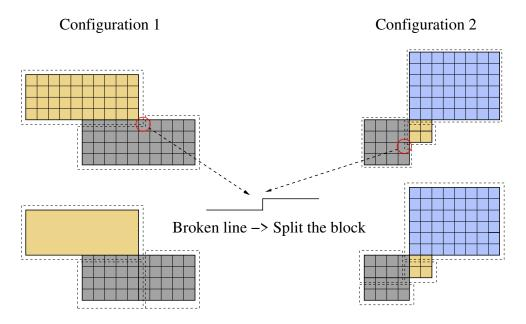
Figure 7.7: Block merging rules.
