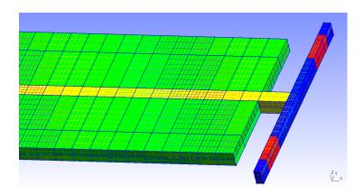
Figure 9.4: Grid of the module for UM2 (27776 elements).
