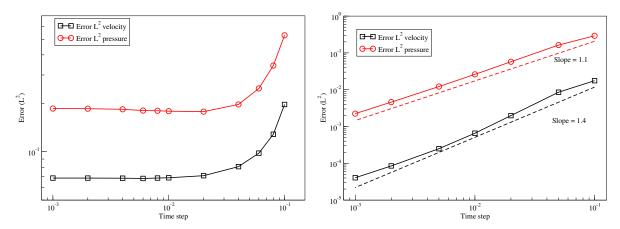
Figure 5.3: Time convergence rates with the standard incremental scheme (left) and the rotational scheme (right) at  $t^* = 1$  with K = 1 and p = 18 with standard open boundary conditions and spectral element method.
