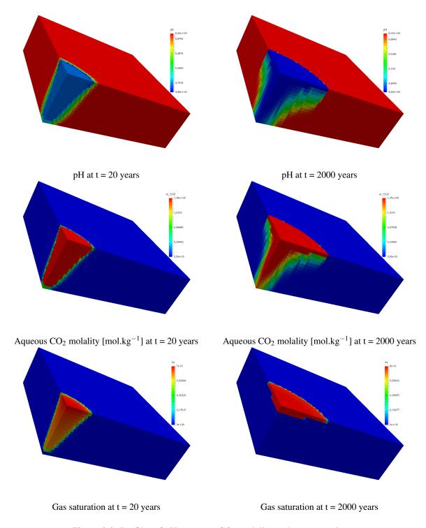
Figure 9.8: Profiles of pH, aqueous CO<sub>2</sub> molality and gas saturation.
