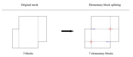
Figure 7.3: Elementary block splitting.
