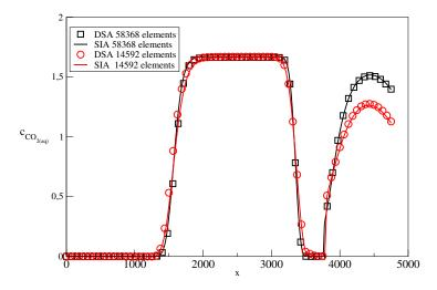
Figure 9.14: Comparison of the concentration of  $CO_{2(aq)}$  obtained with DSA and SIA.
