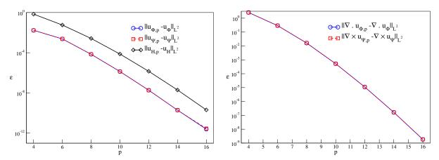
Figure 4.4:  $(L^2(\Omega))^2$ -norm of the error as a function of the polynomial degree p.
