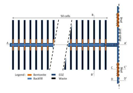
Figure 9.2: Schematic representation of the module (from [304]).
