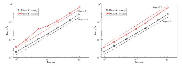
Figure 5.2: Time convergence rates with the standard incremental scheme (left) and the rotational scheme (right) at  $t^* = 1$  with K = 1 and p = 18 with the proposed open boundary conditions and spectral element method.
