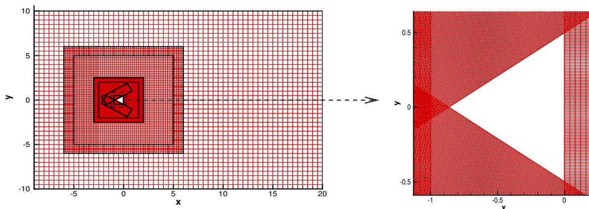
Figure 6.6: Block-structured mesh for the flow past a triangular cylinder.
