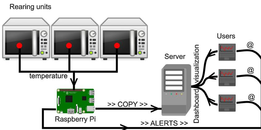
**Fig. 2.** Schematic representation of the monitoring system.
