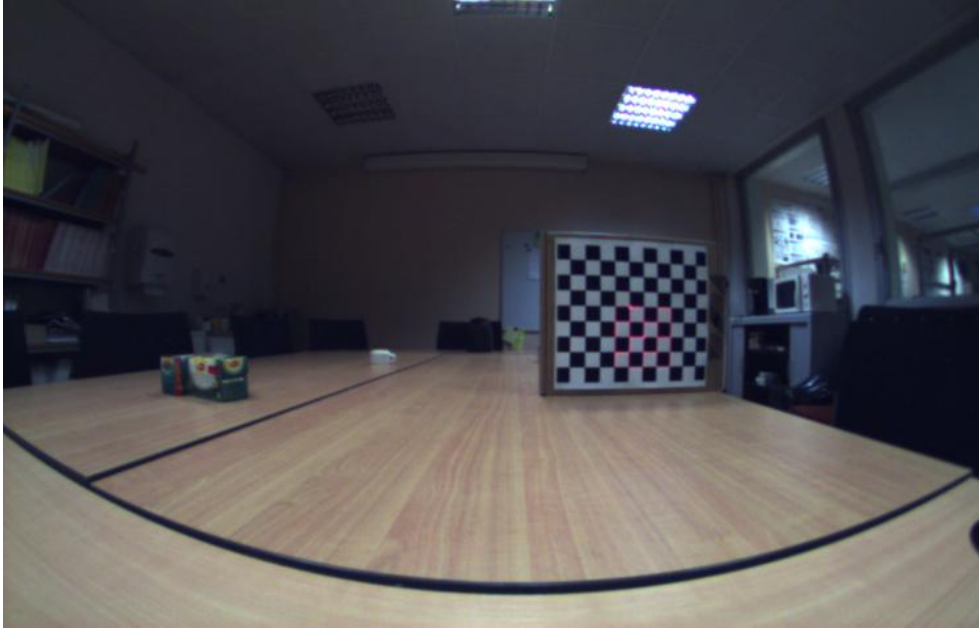
Figure 4.5: The steps to verify for the optical axis of the camera and laser are aligned to each other, it confirms the rotation between the two to be identity.
