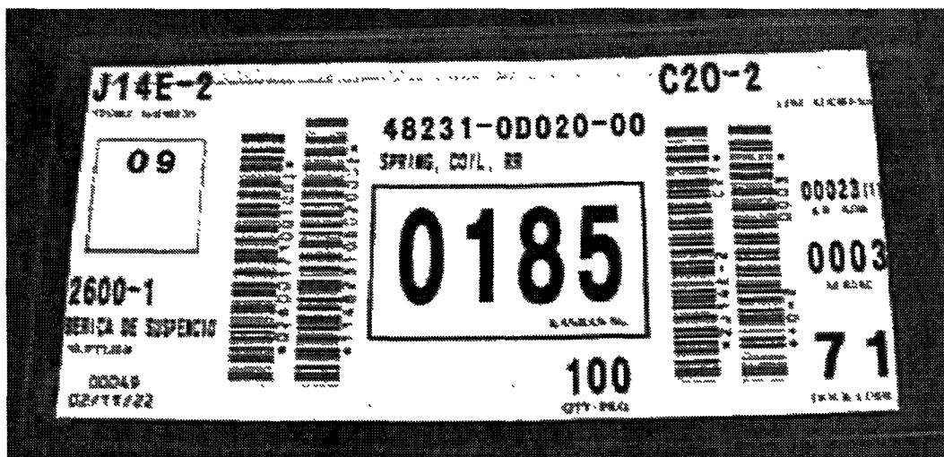
Figure 6-4: Kanban including details of part number, description, designated storage area, standard pack quantity, etc
