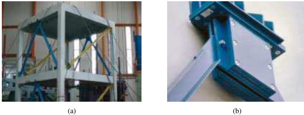
Figure 1.17: Elastomeric viscoelastic dampers [FIP Industrial, 2016]: a) Vibrating table tests on a concrete frame with Elastomeric viscoelastic dampers on top of a reverse V bracing; b) An elastomeric viscoelastic damper installed at the Gentile-Fermi school of Fabriano, Italy.
