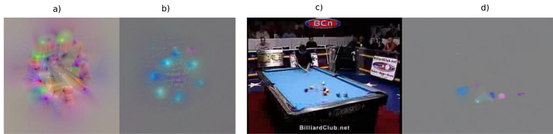
FIGURE 2.26 – Studying a single filter at layer conv5 fusion : (a) and (b) show what maximizes the unit at the input : multiple coloured blobs in the appearance input (a) and moving circular objects at the motion input (b). (c) shows a sample clip from the test set, and (d) the corresponding optical flow (where the RGB channels correspond to the horizontal, vertical and magnitude flow components respectively). Picture credit for [175].
