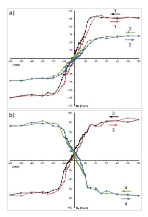
Fig. III.34. (a) Hysteresis loops of the  $B_x$  component extracted from Fig. III.35 (middle column) at position (1) and (2), (b) Hysteresis loops of the  $B_y$  component extracted from Fig. III.35 (right column) at position (3) and (4).
