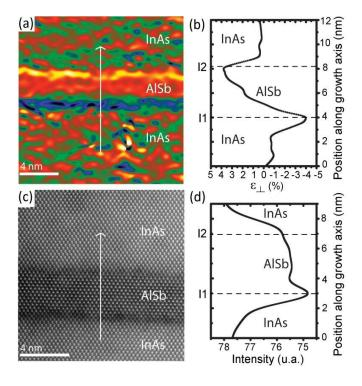
Fig. II.3. (a)  $\varepsilon_{\perp}$  strain map from GPA of an [110] zone axis HRTEM image, (b)  $\varepsilon_{\perp}$  strain profile averaged on the whole width of the image (30 nm), (c) HAADF-STEM micrograph obtained on the same area, (d) Intensity profile from HAADF image plotted along the growth
