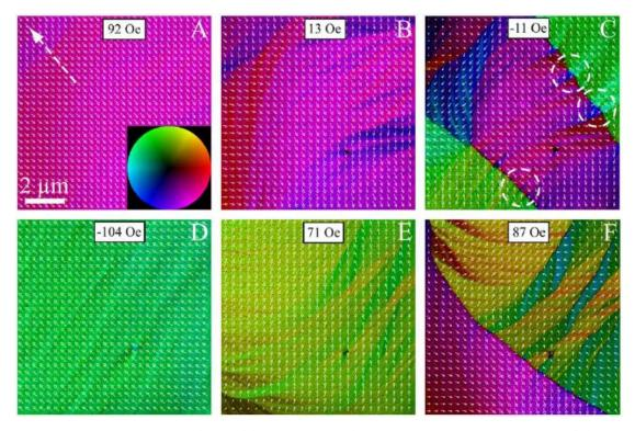
**Fig. III.5.** Six magnetic maps obtained by SIDPC on the  $Co_{35}Fe_{65}(70 \text{ nm})/NiMn(50nm)$  bilayer. On image (A) the unidirectional anisotropy direction is represented by the dashed white arrow. The inserted color wheel indicates the direction of magnetization by the color and the intensity corresponds to the strength of the magnetic signal. On image(C) some cross-tie walls are surrounded.
