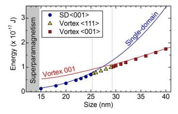
Fig. III.19. Calculated magnetic energy of ferromagnetic iron nanocubes (including a  $1 \text{nm } Fe_3O_4 \text{ shell}$ ) as a function of the total cube size (range 15-40 nm). The energies were calculated once the SD or V configurations were reached. Comparison between random (dots) and frozen SD (blue line) or Vortex <001> (red line) initial states is reported.
