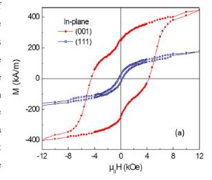
**Fig. II.7.** In-plane magnetic hysteresis loops at 300K of a  $CoFe_2O_4$  (5 nm) film grown on  $MgAl_2O_4$ (100) and  $MgAl_2O_4$ (111).
