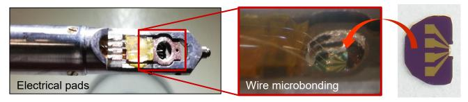
Fig. P.2. Electric connections between the specimen and the sample-holder GATAN HC3500
