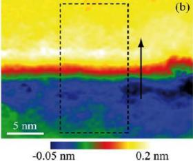
Fig. II.1. (a) HRTEM image of 15 MLs of InAs in [110] zone axis; (b) GPA map of the displacements parallel to the growth axis (spatial resolution of 2 atomic planes). The arrow indicates the growth direction.
