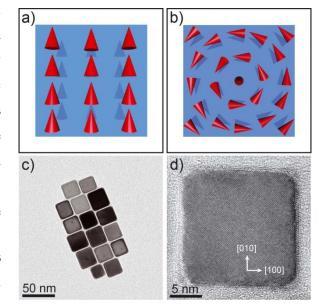
Fig. III.15. Schematic 2D view of (a) a single-domain and (b) a vortex spin arrangement in a square magnetic element. (c) Transmission electron microscopy (TEM) micrograph of Fe nanocubes. (d) High resolution TEM micrograph of a single Fe nanocube.
