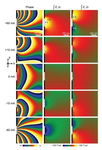
Fig. III.35. Left column: Experimental phase image of the magnetic flux recorded in front of the write pole for an applied current of +60 mA, +10 mA, 0 mA, -10 mA and -60 mA. Middle column: Corresponding  $B_x$  components map integrated over the beam path. Right column: Corresponding  $B_y$  components map integrated over the beam path. The white rectangle on the middle left side of each image is the write pole location.
