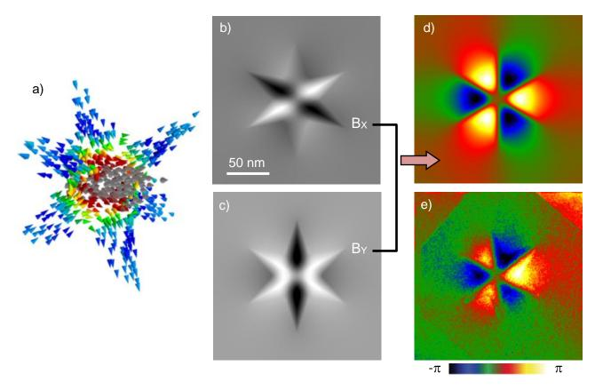
**Fig. III.14.** (a)3D micromagnetic simulation of the FeCo nanostar presented **Fig. III.7**; (b)and (c) In-plane components of the magnetic induction integrated along the electron path and calculated from (a); (d) Simulated magnetic phase image calculated from (b) and (c); (e) Experimental magnetic phase image (MAG) presented **Fig. III.9**.
