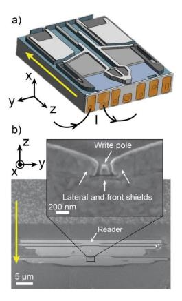
Fig. III.33. (a) Schematic illustration of the HDD slider (I corresponds to the injected current), (b) High magnification SEM image of the read/write parts with a zoom of the write pole inset. The yellow arrows indicate the flying direction of the magnetic media and the electron path for TEM experiments.
