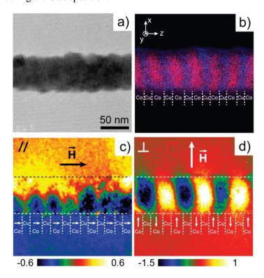
Fig. III.22. (a) TEM image of a  $Co_{25 nm}/Cu_{15 nm}$  nanowire. b) EFTEM image of the same area to distinguish the copper (blue) and cobalt (red) layers. c) Magnetic phase shift map obtained after the application of the parallel saturation field with respect to the wire axis. d) Magnetic phase shift map obtained after the application of the saturation field perpendicularly to the wire axis.
