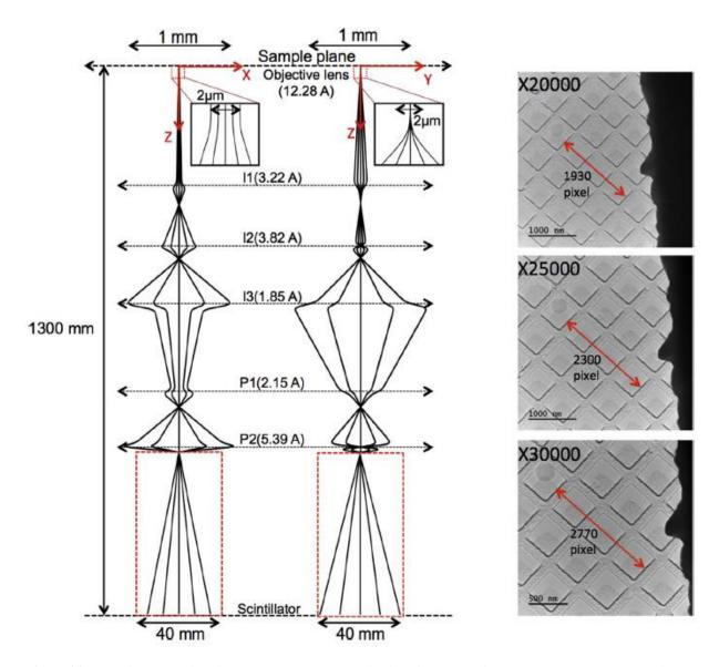
Fig. P.22. Simulation of the electrons trajectories calculated for an arbitrary magnification of 25kX at 300 kV. Only the imaging part of the I2TEM column, in (x,z) and (y,z) planes, is displayed. The images of a cross-grating calibration sample obtained for 20kX, 25kX and 30kX are also reported. The pixel size of the used one-view camera is 15  $\mu$ m.
