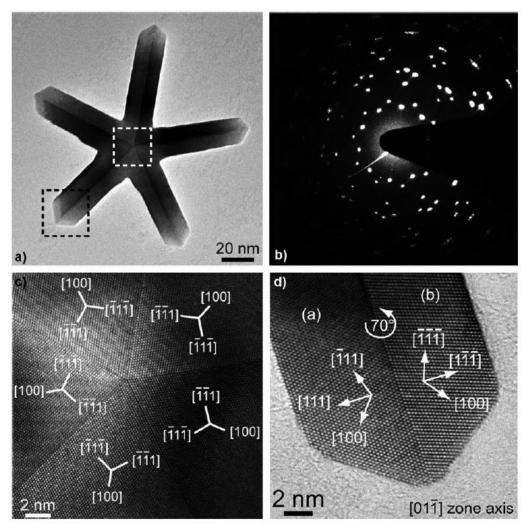
**Fig. II.17.** (a) TEM micrograph of a single Pt fivefold star and (b) its corresponding selected area electron diffraction pattern. HRTEM images of (c) the core and (d) a branch tip as shown in (a) by white and black boxes, respectively.
