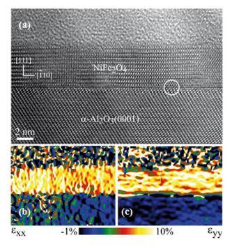
**Fig. II.5.** Cross-sectional HRTEM image of a α-Al2O<sub>3</sub>//NiFe<sub>2</sub>O<sub>4</sub>(111) (5nm) film viewed along the [11-2] zone axis. The circle corresponds to the presence of a misfit dislocation. (b) and (c) Strain maps along the growth direction calculated from the HRTEM image using the GPA method for the (b) in-plane ( $\varepsilon_{xx}$ ) and (c) out-of-plane ( $\varepsilon_{yy}$ ) deformation.
