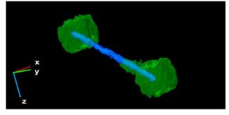
Fig. II.14. 3D representations of the reconstructed volume of a Co-Fe heterostructure using EDX tomography, revealing the distribution of the elements. The segregation between Fe and Co is clearly observed, and that Co nanorod is interlinked with the Fe cubes.
