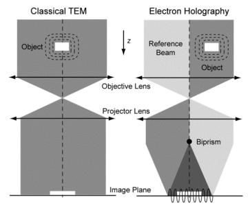
Fig. III.6. Conventional TEM and off-axis EH schemes.
