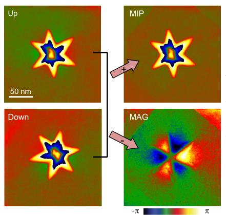
Fig. III.9. Separation of the mean inner potential (MIP) and magnetic (MAG) contributions to the phase shift. MIP and MAP images result of the half sum or half subtraction respectively of up and down observations after switching the sample and numerical alignment.
