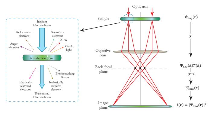
**Fig. 1.1**. Left: signals generated by the electron beam-specimen interaction. Right: basic schematic representation of the image formation by the objective lens in a TEM. Red lines represent the optical path followed by the electrons during the image formation process.
