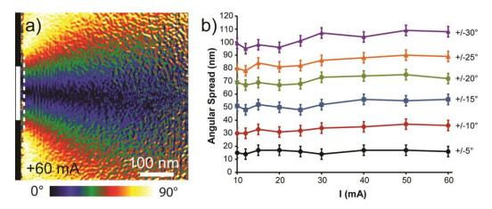
Fig. III.37. (a) Angular spread of the magnetic flux observed for an applied current of +60 mA, (b) Variation of the radiated region width at 5 nm in front of the pole (dashed line in (a) as a function of the applied current and for various flux divergences..
