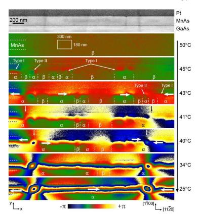
**Fig. III.31.** On the top amplitude image of the studied area; below are displayed the magnetic phase shift maps of the same area at various temperatures in the cooling process. The MnAs layer is between horitonzal dashed line at left of each image. Positions and width of the  $\alpha$  and  $\beta$  domains are denoted. The horizontal white arrows indicate the magnetic induction directions of  $\alpha$  Type- I domains in the MnAs layer.
