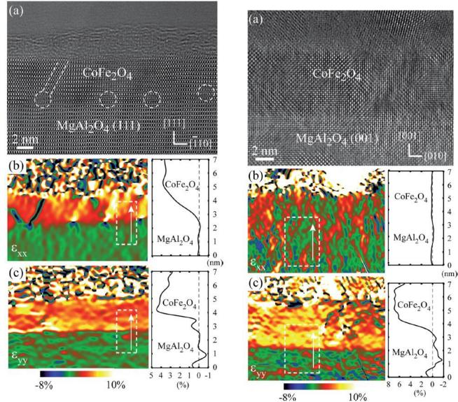
Fig. II.8. HRTEM image of a CoFe2O4(111) film on MgAl2O4(111) (a). Dashed circles indicate dislocations, and the parallel dashed lines mark an antiphase boundary. GPA method applied for the inplane deformation  $\varepsilon_{xx}$  (b) and the out-of-plane deformation  $\varepsilon_{yy}$  (c). Profile of the deformation in dashed rectangle is reported for each direction.
