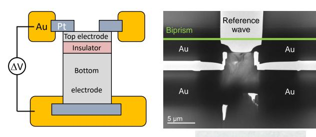
**Fig. P.5.** New geometry proposed for operando experiment of a nanocapacitor. The pre-thinned nanocapacitor is electrically connected to the Au pads of on a  $Si_3N_4$  grid before a final thinning where the  $Si_3N_4$  layer is removed. The biprism (green line) is placed above the upper electrode, the reference wave passing in a field-free area.
