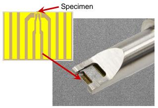
Fig. P.3. Head of the Hummingbird holder with direct insertion of chips. The specimen is mounted on the chip with Au pads.
