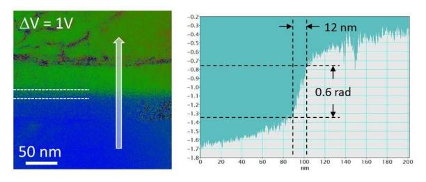
Fig. P.11. Left side: Zoom of the phase image of the electrostatic contribution extracted from the red rectangle in Fig. P.10. The spatial resolution is equal to 0.8 nm. Right side: phase profile extracted from the arrow on the phase image.
