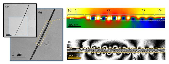
**Fig. III.25.** (a) BF-TEM image and (b) over-focused Lorentz image of sample NW. (c) unwrapped magnetic phase shift image of stippled region marked in (b), and (d) magnetic flux lines obtained from the cosine of (c) with amplification factor 4.
