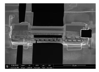
Fig. P.9. Scanning electron micrograph of a connected device by FEBID to Au pads of the Si<sub>3</sub>N<sub>4</sub> membrane.
