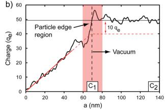
Fig. III.38. (a) Reconstructed phase image of a MgO nanocube; (b) by contour enclosed charge as a function of the short side a; the linear fit of contours within the particle and the constant fit outside of the particle are indicated by red and black lines.
