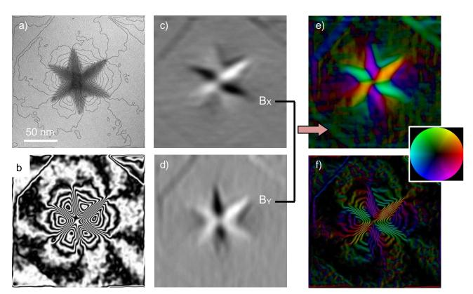
**Fig. III.10.** (a) Isophase lines parallel to induction lines calculated from MAG (**Fig. III.9**). The step between the isophase lines is equal to 0.09 rad. (b) Cosine of MAG with an amplified factor of 15. (c) and (d) X and Y components of the MAG calculated using **Eq. III.9**. (e) Vector map calculated from (c) and (d). The color and its intensity give respectively the direction and the amplitude of the field as seen on the color wheel. (f) Combination of (b) and (e).
