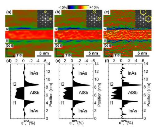
**Fig. II.4.** Out-of-plane strain  $\varepsilon_{\perp}$  maps from a high resolution image with spatial resolutions of 1 nm (a), 0.7nm (b), and 0.45 nm (c). The diffractograms with the different mask sizes are shown in insets. Corresponding profiles of strain along the growth direction (integrated over the width of the image in the [110] direction) are displayed in (d), (e), and (f), respectively.
