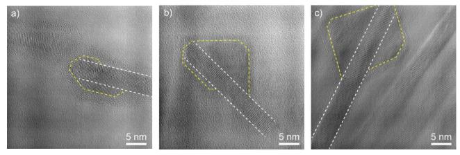
Fig. II.16. HRTEM images of dumbbells at different growth stages.(a) initial Fe deposition close to the Co extremity; (b) growth of a Fe mainly on one side of the nanorod forming a trigonal prism; (c) the growth of the second prism has started.
