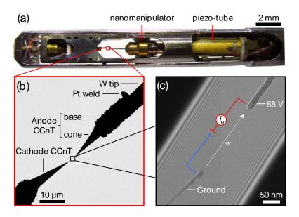
Fig. III.40. (a) Front part of the TEM in situ biasing holder, with the nanomanipulator, driven by a piezo-tube. (b) A zoom-in of the two tips in the holder. c) Further zoom-in and hologram of the two CCnTs, with the top one being biased and the lower one being ground.
