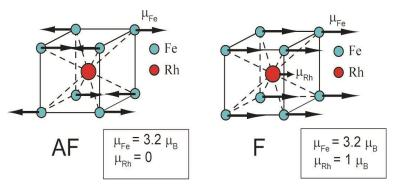
**Fig. II.10.** Scheme of the chemically ordered bcc-phase of  $Fe_{1-x}Rh_x$  B2 phase -AF state for  $T < T_N = 360K$ ; FM state for  $T_N < T < T_C = 680K$ .
