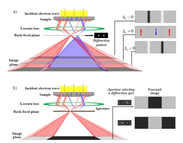
**Fig. III.4.** Schematic representation of the two imaging Lorentz microscopy modes: (a) Fresnel and (b) Foucault modes. Red and yellow arrows located on the sample indicate the magnetization direction of each magnetic domain.
