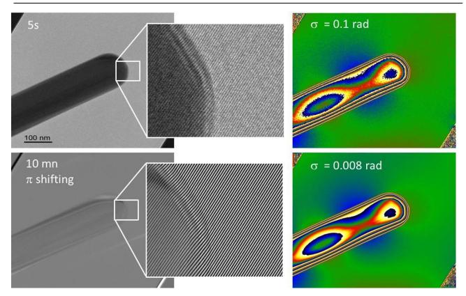
Fig. P.20. Comparison of holograms and corresponding phase images between an usual exposure time of 5 s (top images) and dynamic automation during 10 mn with  $\pi$ -shift method (bottom images). The holograms have been recorded on a magnetic Ni nanowire. The phase noise has been strongly decreased on the  $\pi$ -shifted hologram recorded with 10 mn of exposure time.
