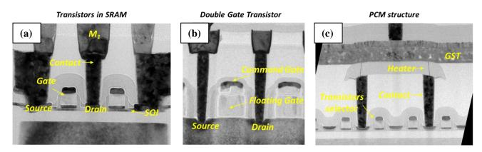
Fig. P.8. Low magnification TEM images of (a) MOSFET transistor, (b) Flash memory cell, and (c) PCM memory.
