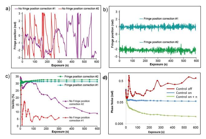
**Fig. P.18.** Fringe stabilization by real-time feedback control of the gun tilts: phase measurements of the fringe position without (a) and with (b) feedback control as a function of the exposure time, and for two acquisition series; (c) and (d) Contrast and phase noise of the corresponding recorded holograms. Note the logarithmic scale for the phase noise.
