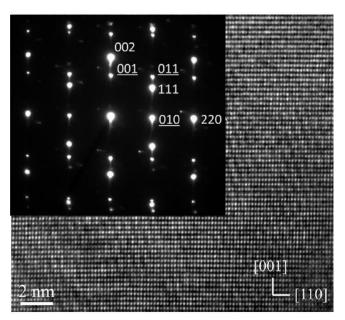
Fig. II.11. HTREM image recorded along the [1-10] zone axis of an equiatomic FeRh layer epitaxially grown on MgO(001). In inset, selected area electron diffraction patterns recorded on the same area showing the chemical order.
