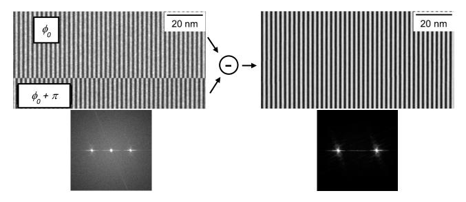
*Fig. P.17.* Principle of  $\square$ -shift method: two  $\square$ -shifted holograms are recorded before being subtracted. The corresponding FFT images show that the auto-correlation term has been removed. The holograms have been acquired using dynamic automation with an exposure time of 5 mn.
