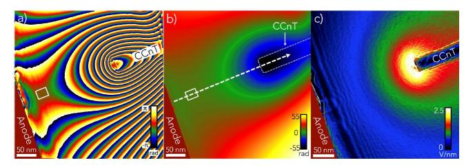
**Fig. III.39.** (a) Experimental phase shift map at 80 V. (b) Unwrapped version of (a). (c) shows the gradient of (b), which represents the integrated electric field (the legend was added only as an indication of the later quantitatively attained field). The white box in (a) and (b) shows the internal reference area.
