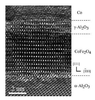
Fig. II.6. HRTEM image of a  $CoFe_2O_4$  (5 nm)/ $\gamma$ - $Al_2O_3$  (1.5 nm)/Co(10 nm) trilayer deposited directly on a sapphire substrate.
