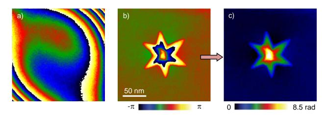
Fig. III.8. (a) Phase image extracted from a reference hologram recorded in vacuum and showing phase distortions coming from the set-up (microscope and camera). (b) Phase image calculated from Fig. III.7.d after subtracting (a). (c) Unwrapped phase image of (b).
