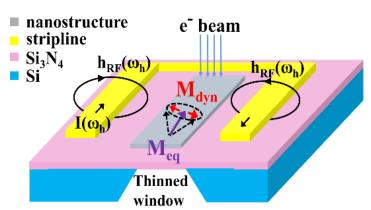
Fig. P.14. Example of sample design for magnonic studies by EH.
