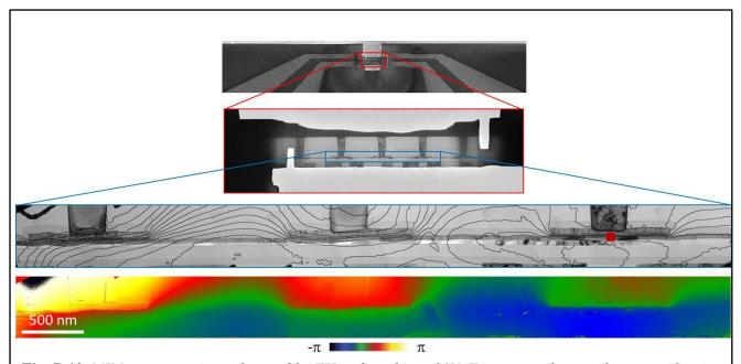
Fig. P.10. MIM nanocapacitors observed by EH under a bias of 1V. From top to bottom: low magnification of the device connected to Au pads of the  $Si_3N_4$  membrane, TEM image of the studied area, amplitude image with isophase contours showing the isopotential lines, phase image used for calculated the contours displayed on the amplitude image.
