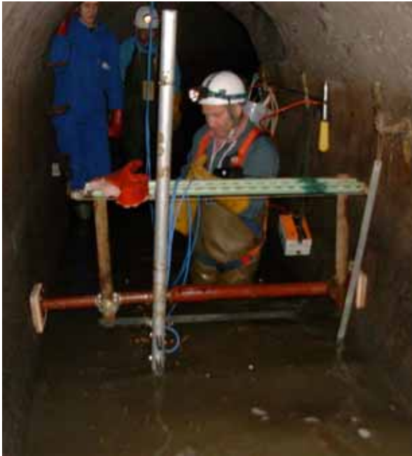
Figure 2. A technician using the fix drop set-up
