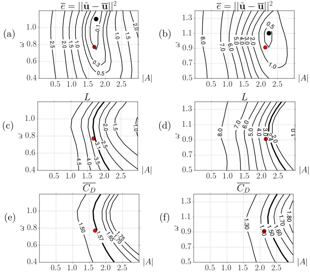
Figure 4.7:  $(\omega, |A|)$  parametric study : (a,b) global error (minimal value marked by a black dot), (c,d) bubble's length and (e,f) mean drag. Results presented for  $Re = 60, 100$ , respectively. Reference (DNS) measured quantities marked in thick line and reference frequency and first-harmonic's amplitude  $(\omega, |A|)$  represented by the red dot.
