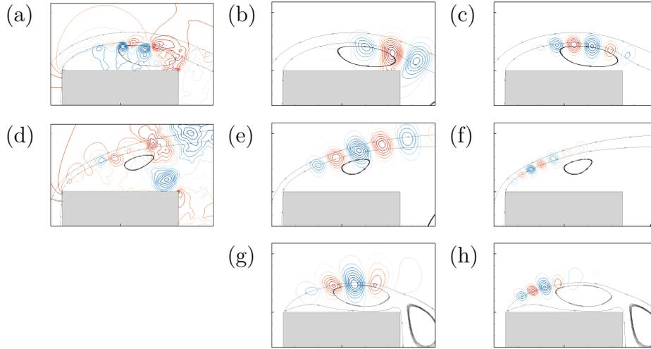
Figure 5.8: Pressure  $p' = p - \langle p \rangle$  snapshots (a,d) at two different phases of the baseline period, corresponding to  $\tau/T = 0$  and  $1/2$  (same phase as in figure 5.7 (a,f,k) and (c,h,m)). The pressure of the modes  $\check{p}$  at those phases are also plotted for  $\omega = 10$  (b,e) and  $\omega = 20$  (c,f). Streamlines correspond to  $\langle \mathbf{u} \rangle$ . Steady-flow modes for  $\omega = 10$  and  $\omega = 20$  are also provided in (g,h) for comparison.
