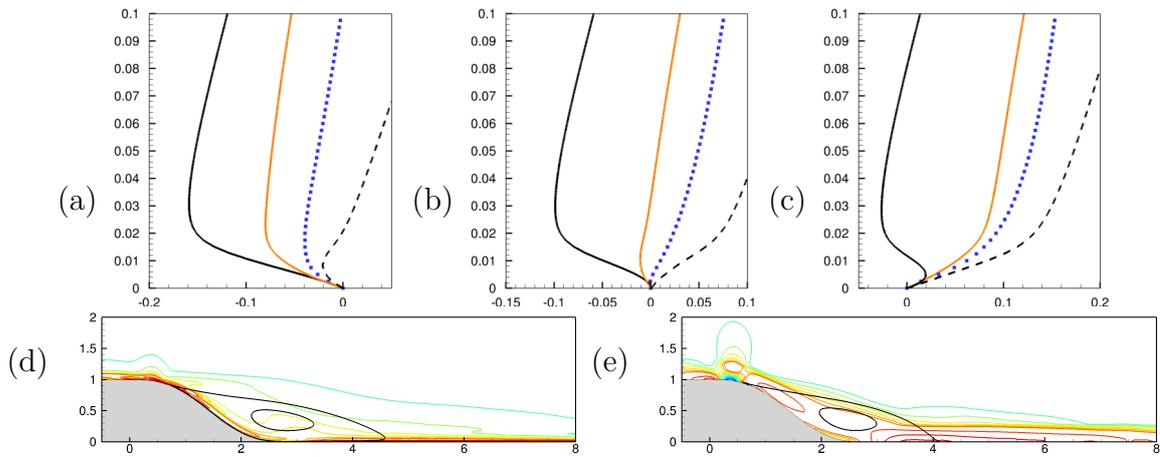
Figure 3.8: Wall-friction assimilation: profiles of  $u_x(y)$  velocity at  $x = 3.5$  (a),  $x = 4$  (b) and  $x = 4.5$  (c). Stream-wise component of the optimal forcing for (d) non-penalized case and (e) penalized case. Black lines represent two streamlines.
