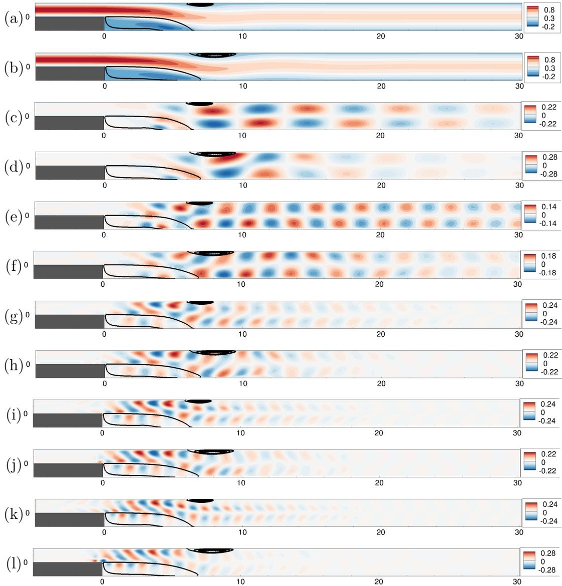
Figure 4.16: Comparison between reconstructed (a,c,e,f,i,k) and reference (b,d,f,h,j,l) fields: mean-flow (a,b) and (normalized) Fourier modes at  $\omega = 0.2$  (c,d),  $\omega = 0.6$  (e,f),  $\omega = 1.0$  (g,h),  $\omega = 1.4$  (i,j),  $\omega = 1.8$  (h,l).
