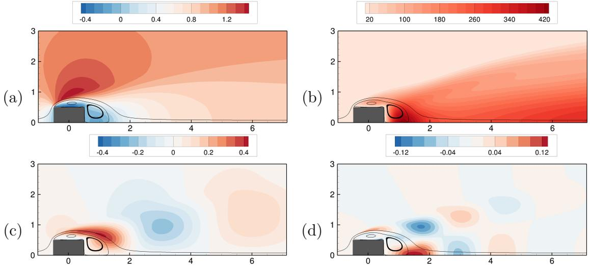
Figure 6.2: URANS solution:  $\bar{U}_x$  mean-velocity field (a), mean-eddy-viscosity  $\tilde{N}/\nu$  (b), first (c) and second (d) harmonic of velocity field. The ratio between their norms is  $|A_0^{URANS}|/|A_1^{URANS}| = 6.7$
