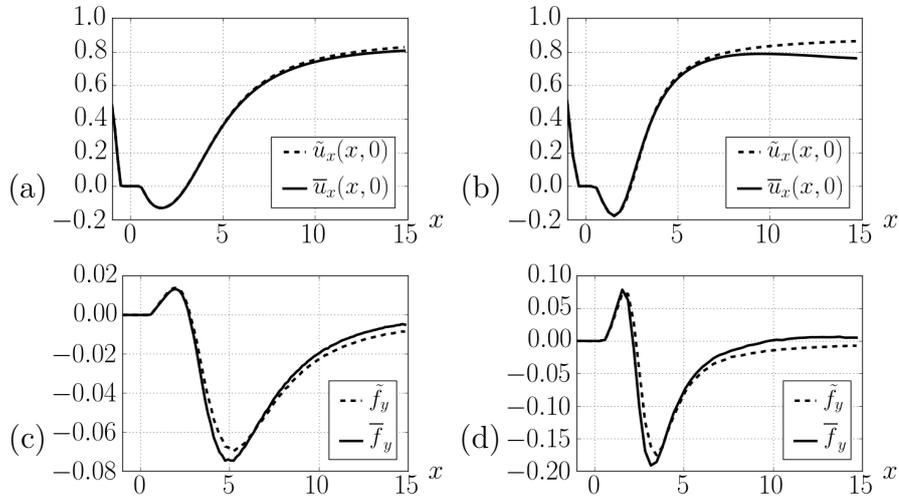
Figure 4.5: Details of reconstructed quantities for  $Re = 60$  (a,c) and  $Re = 100$  (b,d). Mean velocity field (a,b) and Reynolds-stress divergence forcing (c,d)  $\tilde{\mathbf{f}}$  at the centerline  $y = 0$ .
