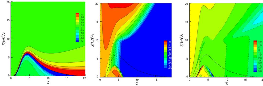
Figure A.1: original SA parameters:  $r$ ,  $s_{PD}$  and its Jacobian  $\partial s_{PD}/\partial\tilde{\nu}$  as function of the two non-dimensional groups  $\chi$  and  $S(\kappa d)^2/\nu$ . The dashed lines on the plots represent the set of parameters for which  $r$  is singular. Figure extracted from Crivellini et al. [2013].
