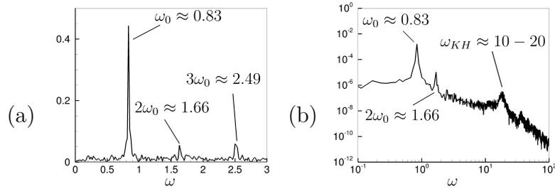
Figure 5.3: DNS: FFT of signal for the (a) cross-wise velocity component at (0, 2.5) (second green dot in figure 5.4) and (b) Power-Spectral Density for the stream-wise velocity on the point (-0.45, 0.63) (first green dot)
