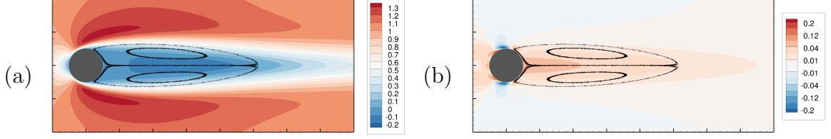
Figure 3.3: Reconstructed velocity field (a) and Reynolds-stress tensor force (b) for wall-pressure assimilation.
