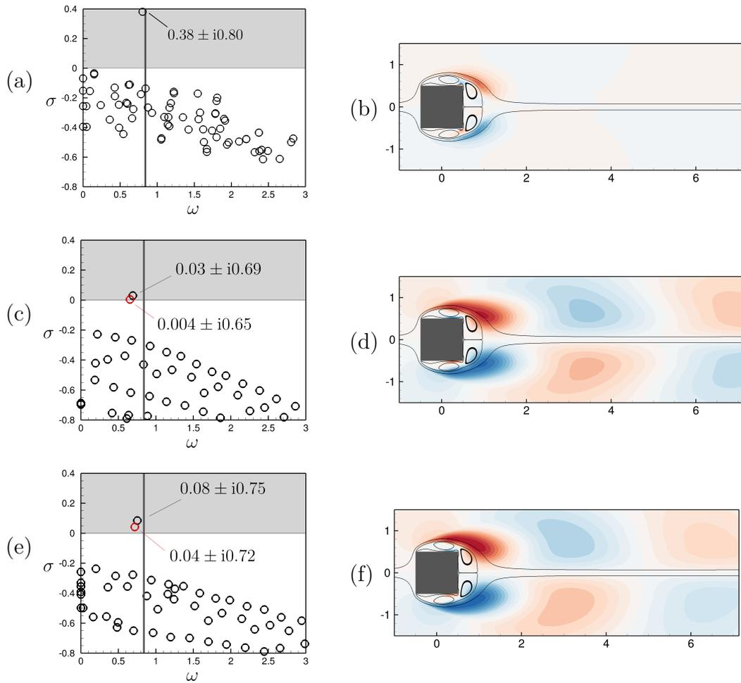
Figure 5.6: Stability analysis: (a,c,e) eigen-spectra and (b,d,f) unstable mode for laminar viscosity approach (a,b), frozen eddy-viscosity (from figure 5.5 (d)) approach (c,d) and variable eddy-viscosity approach (e,f), where  $\tilde{\nu}_t$  is modeled with the Spalart-Allmaras. Red dots correspond to the unstable mode computed from the  $\varepsilon = 0.01$  mean-eddy-viscosity.
