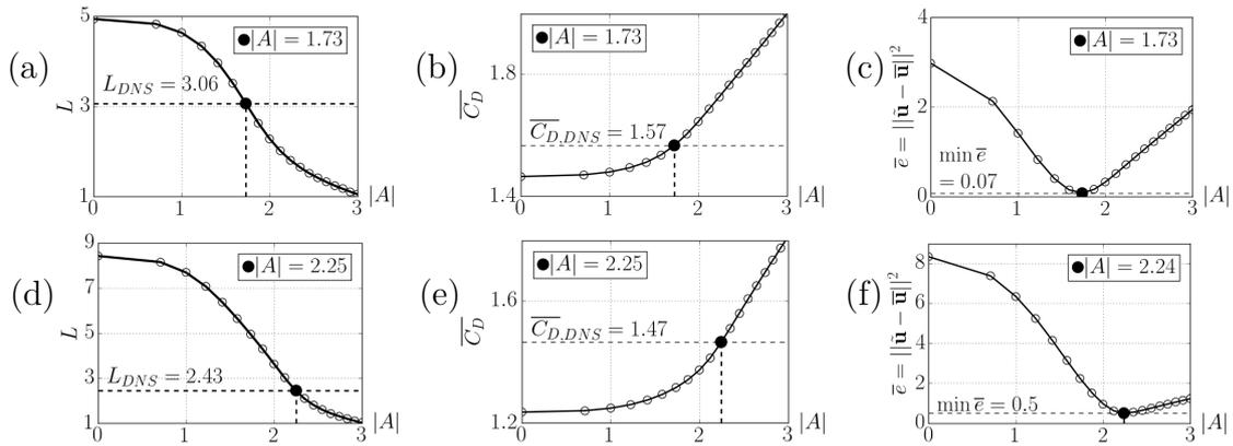
Figure 4.6: Other possible measures: for  $Re = 60$ , we have (a) the length of the recirculation bubble, (b) Mean drag coefficient (c) global error  $\|\tilde{\mathbf{u}} - \bar{\mathbf{u}}\|^2$ . For each different measure, we may have a different (but close) value of the estimated  $|A|$ . Idem for  $Re = 100$ , (b,d,f).
