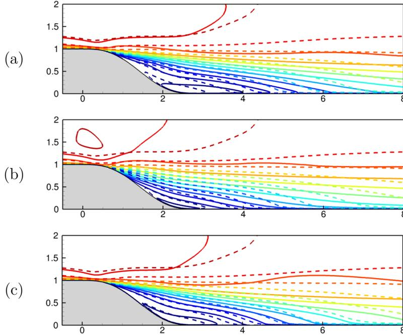
Figure 3.7: Wall-friction assimilation:  $u_x$  iso-contours for model 1 (a), model 2 (b) and  $\gamma = 1$  penalized model 1 (c).
