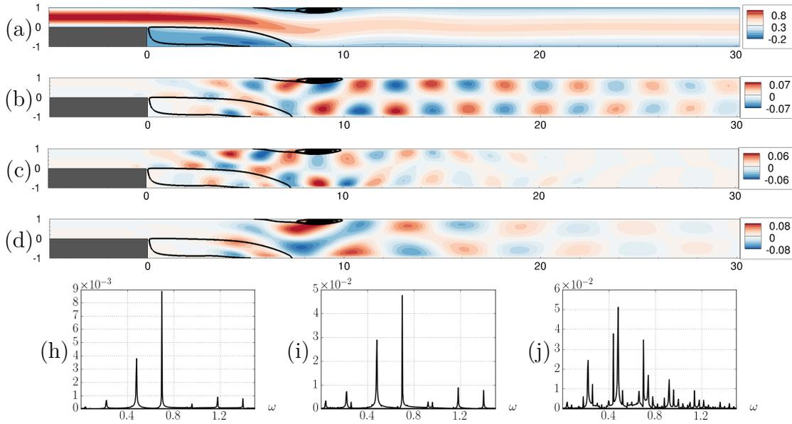
Figure 4.9: (a) Exact time-averaged flow (with  $L = 7.5$ ,  $x_d = 5.8$  and  $x_r = 10.4$ ), (b) Fourier mode at  $\omega = 0.48$ , (c) at  $\omega = 0.70$ , (d) at  $\omega = 0.70 - 0.48 = 0.22$  and spectrum of the cross-velocity-spectra field at (e)  $(x, y) = (1, 0.2)$ , at (f)  $(x, y) = (4, 0.2)$  and (g)  $(x, y) = (15, 0.2)$ .
