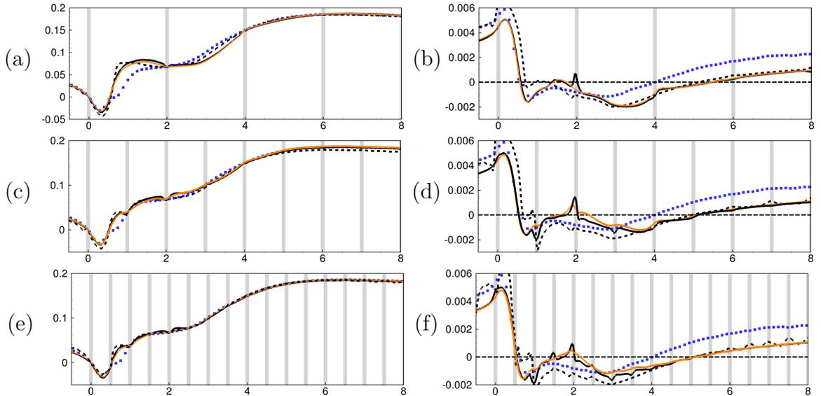
Figure 3.12: Wall-pressure assimilation for three numbers of probes  $N_w = 5, 10$  and  $20$ : wall pressure (a,c,e) and wall-friction (b,d,f). Blue points correspond to the DNS, solid lines correspond to model 1, dashed black lines to the model 2 and orange lines to the model 1 with  $\tilde{\mathbf{f}}_{\mathbf{x}}$ -gradient penalization. The location of pressure measurements are indicated by gray lines.
