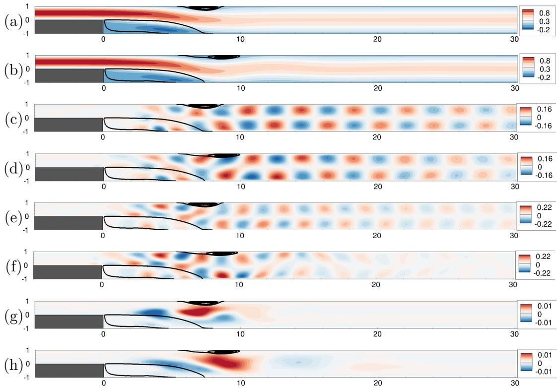
Figure 4.11: Reconstructed fields with optimal parameters  $(|A_1|, |A_2|) = (0.77, 0.44)$  minimizing  $\bar{\epsilon}$ : reconstructed (a) and exact (b) mean flows, reconstructed (normalized) Fourier modes at  $\omega_1 = 0.48$  (c) and (e)  $\omega_2 = 0.7$  and reference ones (d,f). Reynolds stress tensor  $\overline{u'_x u'_y}$  for the model (g) and DNS (h). Identical colour-bars have been used for reconstructed and DNS fields to help comparison.
