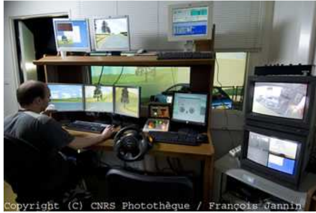
Fig. 47 Control room of UPHF's car driving simulator
