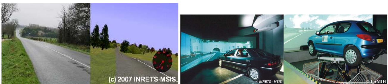
Fig. 70 Evaluation of the impact of perceptual treatment in the field and on two driving simulators: fixed-based one on the left and motion-based one on the right
