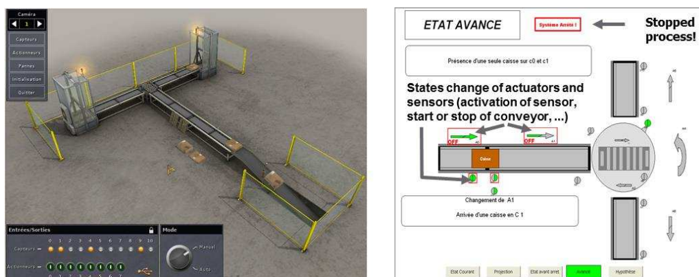
Fig. 80 Experimental platform: ITS-PLC to simulate the operative part of the process (on the left) and the assistance system (on the right) providing explanations about process stop and command errors
