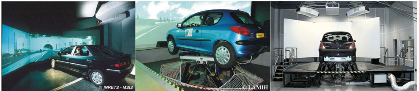
Fig. 37 Driving simulators of IFSTTAR (a static one on left), UPHF-LAMIH (a mobile one) and Renault (mobile one on the right)
