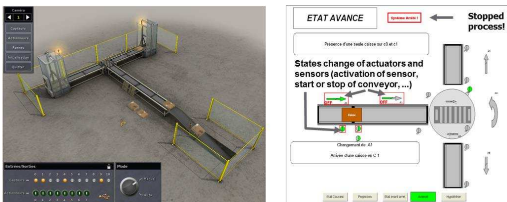
Fig. 80 Experimental platform: ITS-PLC to simulate the operative part of the process (on the left) and the assistance system (on the right) providing explanations about process stop and command errors
