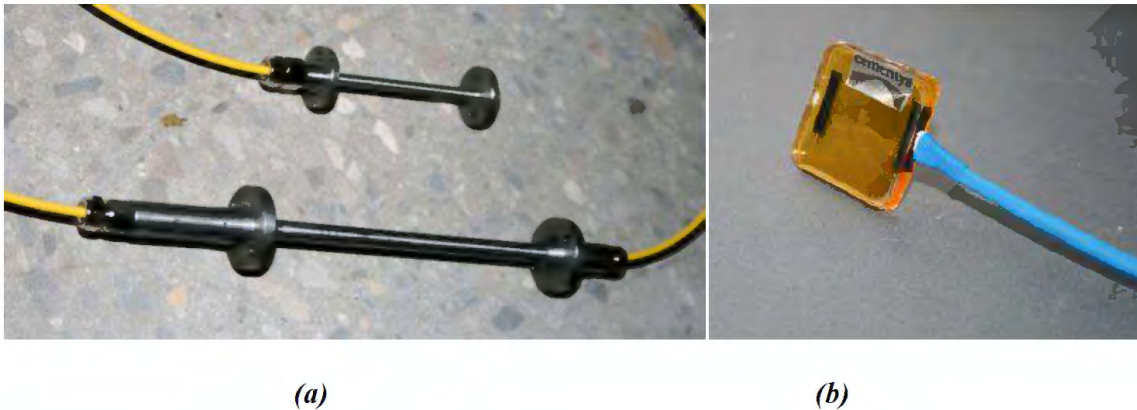
Figure 1-11: Fiber Bragg Grating sensor adapted (a) to be embedded and (b) mounted on the surface for monitoring of civil engineering structures. (Excerpt from CEMENTYS)
