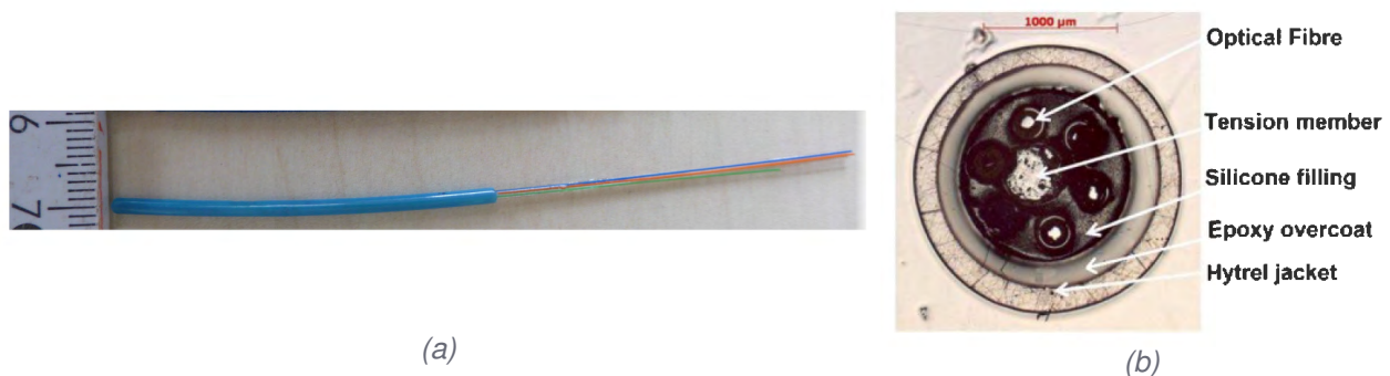
Figure 3-24: (a) Photo of the SensoLux cable. (b) Micrograph of different constitutive layers of SensoLux optical cable [57].
