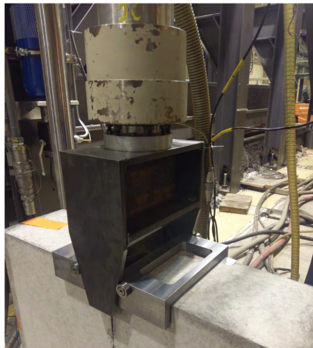
Figure 3-4: Mechanical pieces fabricated for the wedge splitting test.
