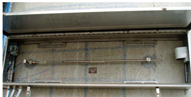
Figure 1-3: LVDT sensors installed on site on the left of a 1 m Invar bar [15].
