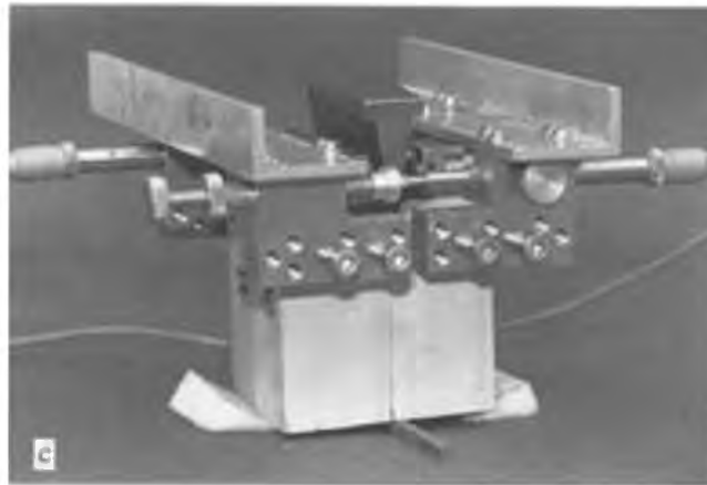
Figure 3-1: First Wedge Splitting Test (WST) configuration proposed by Tschegg in 1986 [141].
