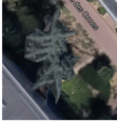
Figure 3.7 – A zoom on Google Maps’ reconstruction of a tree. In this reconstruction, the different branches of the tree are connected together in order to form a simpler polygon which do not represent the original geometry of the scene.
