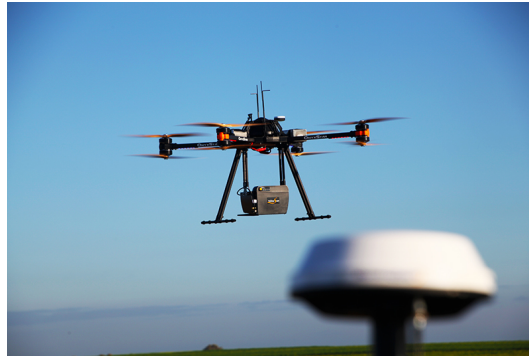
Figure 2.7 – Illustration of a UAV-based LiDAR sensor. Courtesy of Wikipedia Commons.
