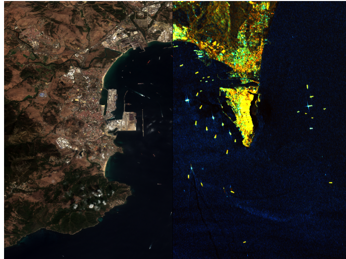
Figure 1.4 – Optical image (left) and Radar image (right) used for ship detection in the Gibraltar straight. The geometric complexity of ships makes them easily identifiable from a Radar point of view. Courtesy of Anatol Garioud (IGN-LaSTIG-STRUDEL).
