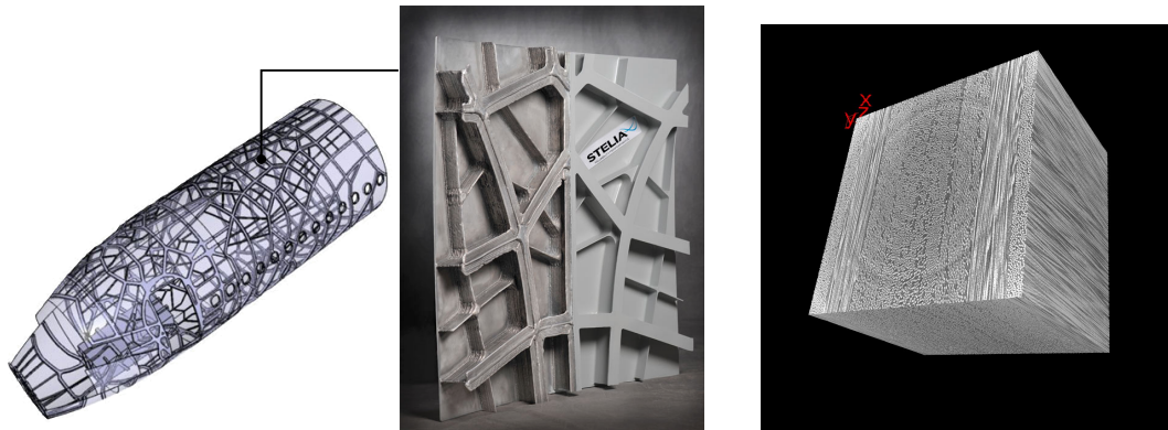
(a) Innovative stiffened structures with curvilinear stiffeners [Renard, 2018].
