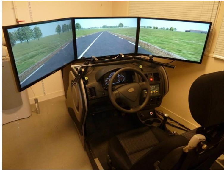
Figure D-1 : Driving simulator setup: the driving scene is displayed on three screens.
