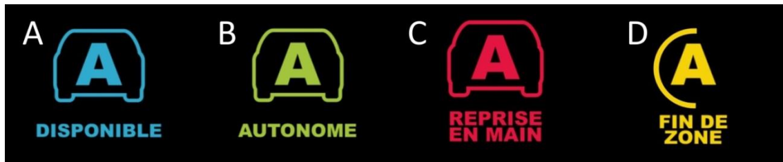
Figure F-2 : Pictograms displayed on the HMI. A, autonomous driving available; B, autonomous driving activated; C, critical take-over request (8s); D, planned take-over request (45s)
