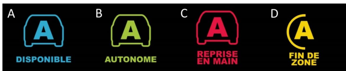
Figure E-2 : Pictograms displayed on the HMI. A: autonomous driving available; B: autonomous driving activated; C: take-over request (8 s); D: take-over request (45 s)
