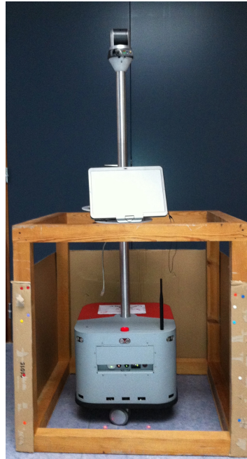
FIGURE 4.5 – Testing the Robot Sensors in a Static Known Environment
