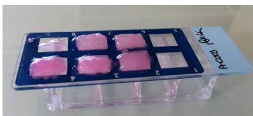
Figure II-19: Typical aspect of 90 min cooled Gal-C7 hydrogels after 7 days of cell culture on an 8-well chamber slide (after chamber removal). The two wells at the right are controls.
