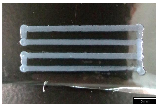
Figure III-29: Example of a printed Gal-C7 hydrogel (2.5 wt % solution, 10 \mu\text{l}/\text{min} , 2 mm/s printing speed, 2 mm between the needle and the membrane). Scale bar: 5 mm.
