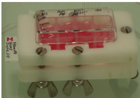
Figure II-18: 8-well chamber slide with the tool used to prepare hydrogels with controlled cooling rate conditions.
