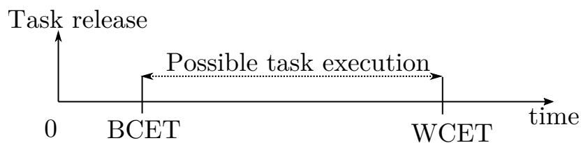
Figure 1.2: Task execution times lies between the BCET and WCET for predictability of task execution.
