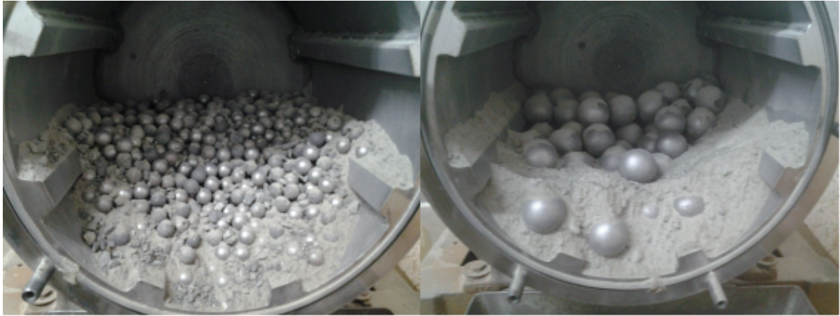
Figure 1.6 – Images of a ball mill with lifters filled with the product and steel balls of two different sizes [88].
