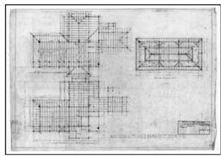
Framing plans: 1F and 2F; Truss plan: 2F (1:50)
