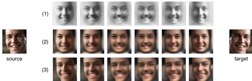
Figure 2.11: Lighting interpolation with Intrinsic-DAE. With latent representations learnt in an unsupervised manner for shading, albedo, and deformation, the DAE allows us to simulate smooth transitions of the lighting direction. In this example, we interpolate the latent representation of the shading from source (lit from the left) to target (mirrored source, hence lit from the right). The network generates smooth lighting transitions, without explicitly learning geometry, as shown in shading (1) and texture (2). Together with the learnt deformation of the source image, DAE enables the relighting of the face in its original pose (3).
