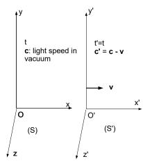
FIGURE 2.1 – Galilean transformation (classical mechanics)
