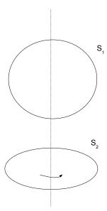
Figure 5.1 – Relative rotation of two fluid masses
